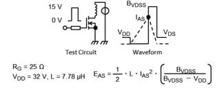
Fig. 8.16 Test Circuit/Waveform
