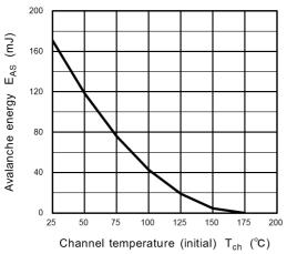
Fig. 8.15 E<sub>AS</sub> - T<sub>ch</sub>(Guaranteed Maximum)
