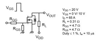
Fig. 6.2.1 Switching Time Test Circuit
