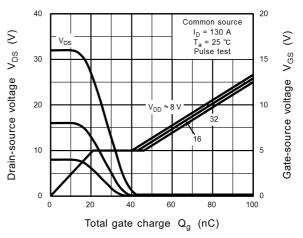
Fig. 8.14 Dynamic Input/Output Characteristics
