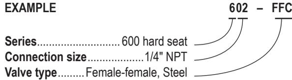
To meet all of your specific application requirements, the following **additional options** are available for these needle valves. To order all or any of these options, simply add them to the part number as shown in the diagram below.
