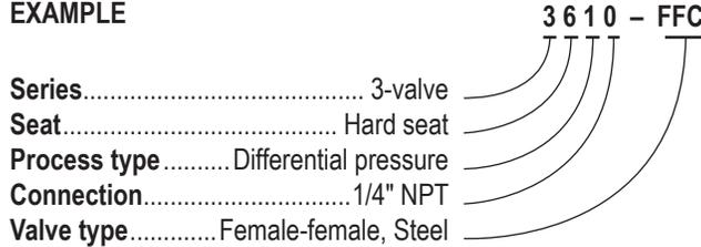
To meet all of your specific application requirements, the following **additional options** are available for these manifold valves. To order all or any of these options, simply add them to the part number as shown in the diagram below.
