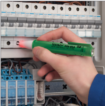
Testboy illuminates with voltage present
