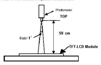
**Note 2:** Measured at the centre area of the panel and at the viewing angle of the  $\theta x = \theta y = 0^{\circ}$
