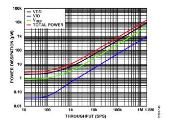
Figure 35. Power Dissipation vs. Throughput
