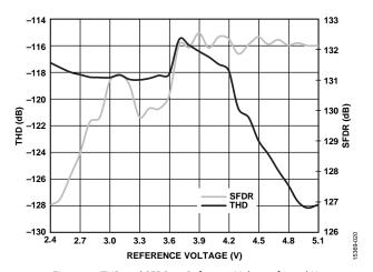
Figure 21. THD and SFDR vs. Reference Voltage,  $f_{\text{IN}} = 1 \text{ kHz}$
