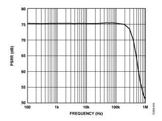
Figure 33. PSRR vs. Frequency
