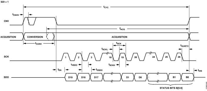
Figure 52. CS Mode, 3-Wire Without Busy Indicator Serial Interface Timing Diagram Including Status Bits
