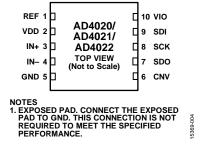
Figure 4. 10-Lead LFCSP Pin Configuration
