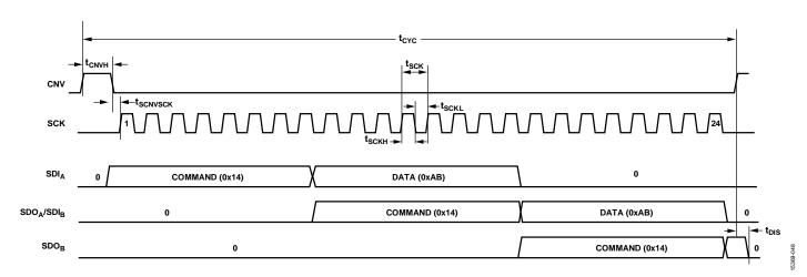
Figure 51. Register Write Timing Diagram, Daisy-Chain Mode
