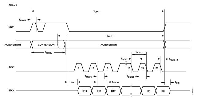
Figure 56. CS Mode, 3-Wire Without the Busy Indicator Serial Interface Timing Diagram (Status Bits Not Shown)
