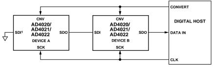
1SDI MUST BE CONNECTED TO THE DIGITAL HOST DATA OUT TO WRITE TO THE CONFIGURATION REGISTER.
