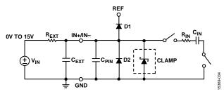
Figure 43. Equivalent Analog Input Circuit
