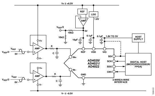
Figure 40. Typical Application Diagram with Multiple Supplies
