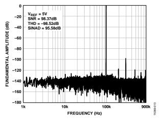
Figure 13. 100 kHz, -0.5 dBFS Input Tone FFT
