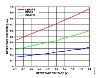
Figure 34. Reference Current vs. Reference Voltage
