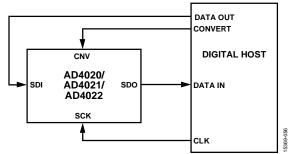
Figure 59. CS Mode, 4-Wire Turbo Mode Connection Diagram
