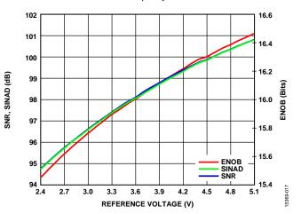
Figure 18. SNR, SINAD, and ENOB vs. Reference Voltage,  $f_{\text{IN}} = 1 \text{ kHz}$
