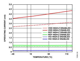
Figure 30. Operating Current vs. Temperature, AD4021, 1 MSPS
