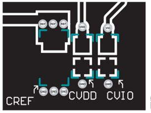
Figure 68. Example Layout of the AD4020 (Bottom Layer)
