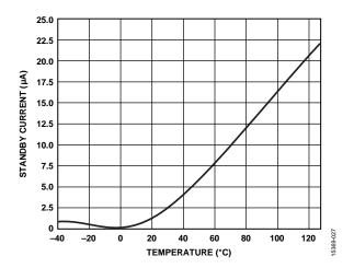
Figure 36. Standby Current vs. Temperature
