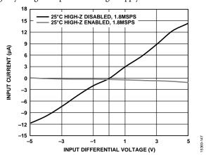
Figure 2. Input Current vs. Input Differential Voltage
