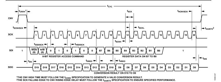
Figure 50. Register Write Timing Diagram
