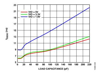
Figure 37. t<sub>DSDO</sub> vs. Load Capacitance
