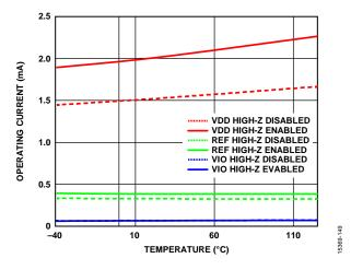
Figure 31. Operating Current vs. Temperature, AD4022, 500 kSPS
