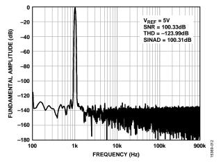
Figure 12. 1 kHz, -0.5 dBFS Input Tone Fast Fourier Transform (FFT),  $V_{occ} = 5 V$
