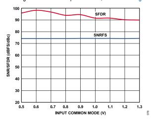
Figure 54. SNR/SFDR vs. Input Common-Mode Voltage, f<sub>IN</sub> = 9.7 MHz, f<sub>SAMPLE</sub> = 125 MSPS
