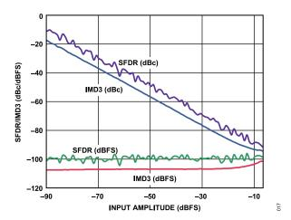
Figure 19. Two-Tone SFDR/IMD3 vs. Input Amplitude (AIN) with  $f_{\rm IN1}$  = 70.5 MHz and  $f_{\rm IN2}$  = 72.5 MHz,  $f_{\rm SAMPLE}$  = 80 MSPS
