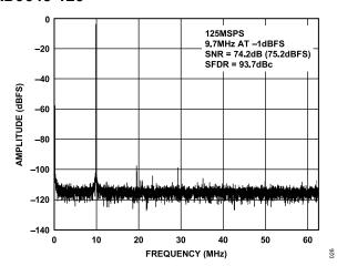
Figure 28. Single-Tone 16k FFT with  $f_{\rm IN}$  = 9.7 MHz,  $f_{\rm SAMPLE}$  = 125 MSPS
