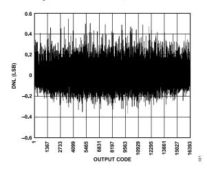
Figure 23. DNL;  $f_{IN}$  = 9.7 MHz,  $f_{SAMPLE}$  = 80 MSPS
