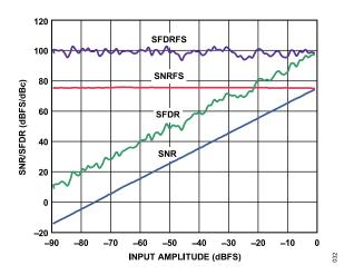
Figure 34. SNR/SFDR vs. Analog Input Level;  $f_{\rm IN}$  = 9.7 MHz,  $f_{\rm SAMPLE}$  = 125 MSPS
