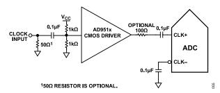
Figure 63. Single-Ended 1.8 V CMOS Input Clock (Up to 200 MHz)
