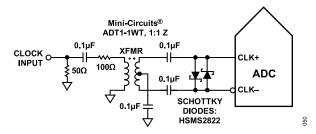
Figure 59. Transformer-Coupled Differential Clock (Up to 200 MHz)
