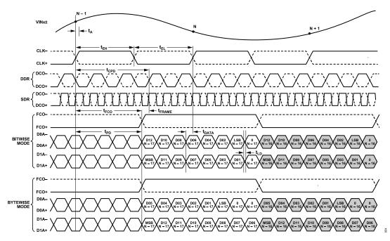
Figure 4. 16-Bit DDR/SDR, Two-Lane, 2× Frame Mode
