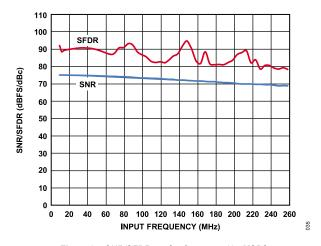
Figure 37. SNR/SFDR vs.  $f_{IN}$ ;  $f_{SAMPLE} = 125 MSPS$
