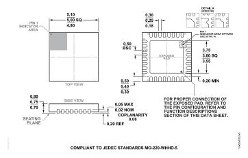
Figure 72. 32-Lead Lead Frame Chip Scale Package [LFCSP] 5 mm × 5 mm Body and 0.75 mm Package Height (CP-32-12) Dimensions shown in millimeters
