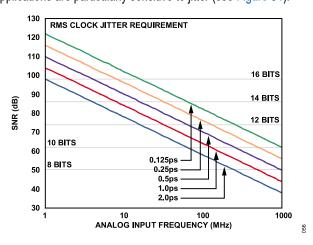
Figure 64. Ideal SNR vs. Input Frequency and Jitter
