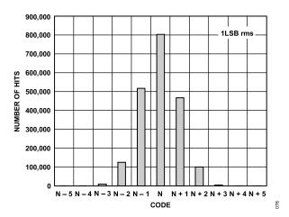
Figure 41. Input Referred Noise Histogram; f<sub>SAMPLE</sub> = 125 MSPS
