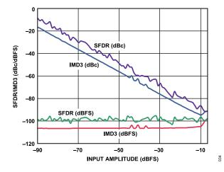
Figure 36. Two-Tone SFDR/IMD3 vs. Input Amplitude (AIN) with  $f_{\rm IN1}$  = 70.5 MHz and  $f_{\rm IN2}$  = 72.5 MHz,  $f_{\rm SAMPLE}$  = 125 MSPS
