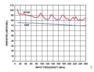
Figure 20. SNR/SFDR vs.  $f_{IN}$ ;  $f_{SAMPLE} = 80$  MSPS
