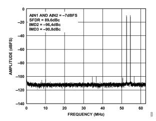
Figure 35. Two-Tone 16k FFT with  $f_{\rm IN1}$  = 70.5 MHz and  $f_{\rm IN2}$  = 72.5 MHz,  $f_{\rm SAMPLE}$  = 125 MSPS
