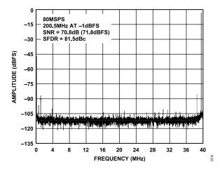
Figure 16. Single-Tone 16k FFT with  $f_{\rm IN}$  = 200.5 MHz,  $f_{\rm SAMPLE}$  = 80 MSPS, Clock Divide = Divide-by-8
