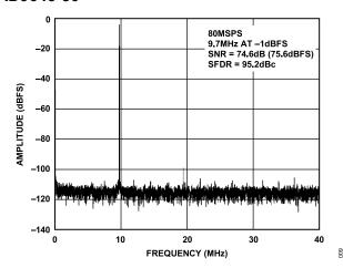
Figure 9. Single-Tone 16k FFT with  $f_{\rm IN}$  = 9.7 MHz,  $f_{\rm SAMPLE}$  = 80 MSPS
