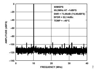
Figure 12. Single-Tone 16k FFT with  $f_{\rm IN}$  = 69.5 MHz,  $f_{\rm SAMPLE}$  = 80 MSPS, Temp = -40  $^{\circ}$ C
