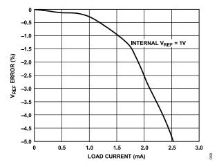
Figure 57. V<sub>REF</sub> Error vs. Load Current
