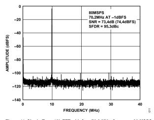
Figure 11. Single-Tone 16k FFT with  $f_{\rm IN}$  = 70.2 MHz,  $f_{\rm SAMPLE}$  = 80 MSPS
