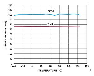
Figure 21. SNR/SFDR vs. Temperature;  $f_{IN}$  = 9.7 MHz,  $f_{SAMPLE}$  = 80 MSPS
