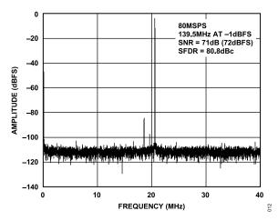
Figure 14. Single-Tone 16k FFT with  $f_{IN}$  = 139.5 MHz,  $f_{SAMPLE}$  = 80 MSPS
