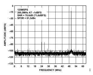
Figure 33. Single-Tone 16k FFT with  $f_{\rm IN}$  = 200.5 MHz,  $f_{\rm SAMPLE}$  = 125 MSPS, Clock Divide = Divide-by-8
