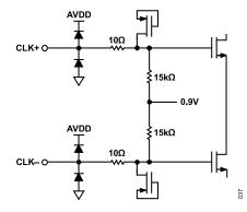
Figure 46. Equivalent Clock Input Circuit
