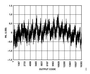
Figure 39. INL;  $f_{IN}$  = 9.7 MHz,  $f_{SAMPLE}$  = 125 MSPS
