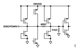
Figure 47. Equivalent SDIO/PDWN Input Circuit
