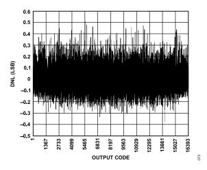
Figure 40. DNL;  $f_{IN}$  = 9.7 MHz,  $f_{SAMPLE}$  = 125 MSPS
