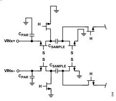
Figure 53. Switched-Capacitor Input Circuit
