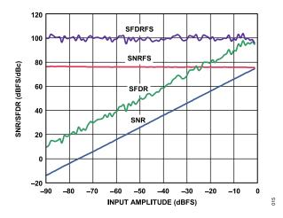
Figure 17. SNR/SFDR vs. Analog Input Level;  $f_{\rm IN}$  = 9.7 MHz,  $f_{\rm SAMPLE}$  = 80 MSPS
