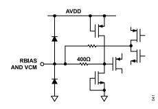
Figure 50. Equivalent RBIAS and VCM Circuit
