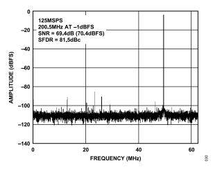
Figure 32. Single-Tone 16k FFT with  $f_{\rm IN}$  = 200.5 MHz,  $f_{\rm SAMPLE}$  = 125 MSPS
