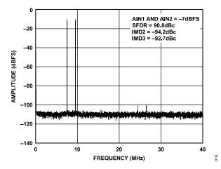
Figure 18. Two-Tone 16k FFT with  $f_{\rm IN1}$  = 70.5 MHz and  $f_{\rm IN2}$  = 72.5 MHz,  $f_{\rm SAMPLE}$  = 80 MSPS
