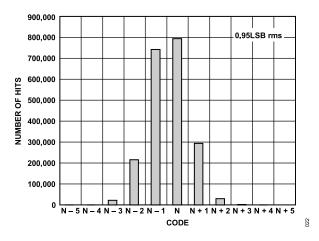
Figure 24. Input Referred Noise Histogram; f<sub>SAMPLE</sub> = 80 MSPS
