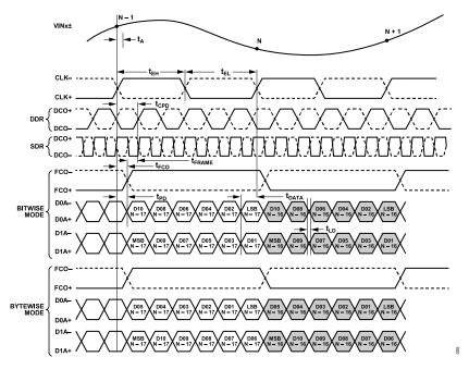
Figure 5. 12-Bit DDR/SDR, Two-Lane, 2× Frame Mode
