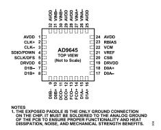
Figure 8. Pin Configuration, Top View
