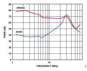
Figure 42. PSRR vs. Frequency;  $f_{CLK}$  = 125 MHz,  $f_{SAMPLE}$  = 125 MSPS
