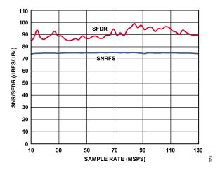
Figure 44. SNR/SFDR vs. Sample Rate;  $f_{\rm IN}$  = 70 MHz,  $f_{\rm SAMPLE}$  = 125 MSPS
