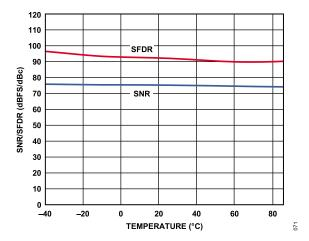
Figure 38. SNR/SFDR vs. Temperature;  $f_{IN}$  = 9.7 MHz,  $f_{SAMPLE}$  = 125 MSPS
