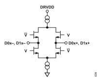
Figure 48. Equivalent Digital Output Circuit
