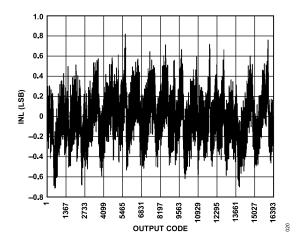
Figure 22. INL;  $f_{IN} = 9.7 \text{ MHz}$ ,  $f_{SAMPLE} = 80 \text{ MSPS}$
