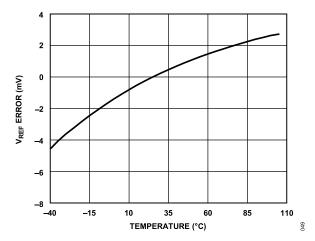
Figure 58. Typical V<sub>REF</sub> Drift
