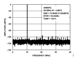
Figure 13. Single-Tone 16k FFT with  $f_{\rm IN}$  = 69.5 MHz,  $f_{\rm SAMPLE}$  = 80 MSPS, Temp = 105  $^{\circ}$ C
