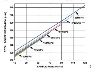
Figure 65. Total Power Dissipation vs.  $f_{SAMPLE}$  for  $f_{IN}$  = 9.7 MHz
