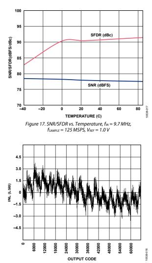
Figure 18. INL,  $f_{IN} = 9.7 \text{ MHz}$ ,  $f_{SAMPLE} = 125 \text{ MSPS}$ ,  $V_{REF} = 1.0 \text{ V}$
