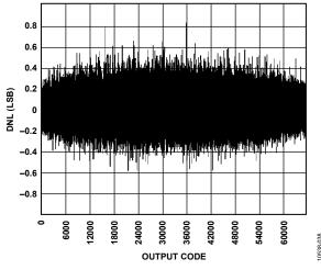
Figure 38. DNL,  $f_{IN} = 9.7 \text{ MHz}$ ,  $f_{SAMPLE} = 125 \text{ MSPS}$ ,  $V_{REF} = 1.3 \text{ V}$
