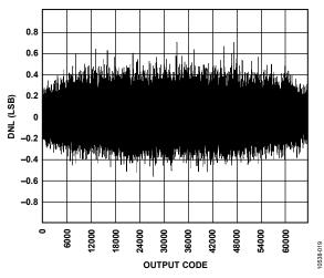
Figure 19. DNL,  $f_{IN} = 9.7 \text{ MHz}$ ,  $f_{SAMPLE} = 125 \text{ MSPS}$ ,  $V_{REF} = 1.0 \text{ V}$
