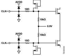
Figure 44. Equivalent Clock Input Circuit
