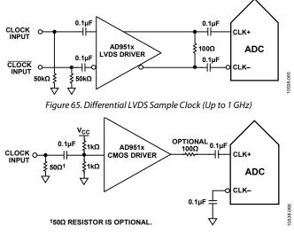
Figure 66. Single-Ended 1.8 V CMOS Input Clock (Up to 200 MHz)
