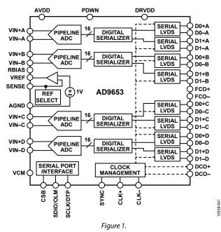
as programmable output clock and data alignment and digital test pattern generation. The available digital test patterns include built-in deterministic and pseudorandom patterns, along with custom user-defined test patterns entered via the serial port interface (SPI).
