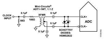
Figure 62. Transformer-Coupled Differential Clock (Up to 200 MHz)
