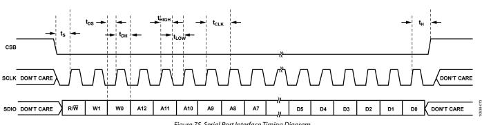
Figure 75. Serial Port Interface Timing Diagram
