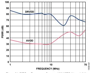
Figure 21. PSRR vs. Frequency, f<sub>SAMPLE</sub> = 125 MSPS, V<sub>REF</sub> = 1.0 V
