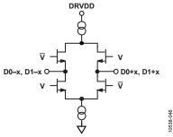
Figure 46. Equivalent Digital Output Circuit
