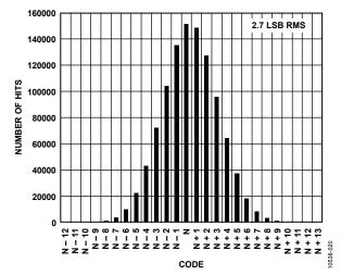
Figure 20. Input-Referred Noise Histogram, f<sub>SAMPLE</sub> = 125 MSPS, V<sub>REF</sub> = 1.0 V
