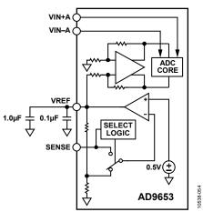
Figure 54. 1.0 V Internal Reference Configuration
