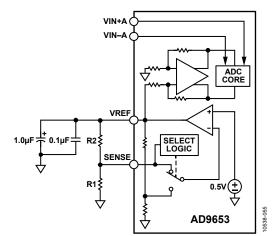
Figure 55. Programmable Internal Reference Configuration
