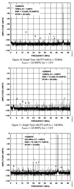
Figure 12. Single-Tone 16k FFT with  $f_{IN} = 200.5$  MHz at  $f_{SAMPLE} = 125$  MSPS,  $V_{REF} = 1.0 V$
