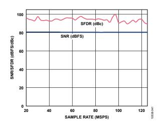
Figure 41. SNR/SFDR vs. Sample Rate,  $f_{IN} = 9.7 \text{ MHz}$ ,  $V_{REF} = 1.3 \text{ V}$
