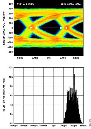
Figure 74. Data Eye for LVDS Outputs in ANSI-644 Mode with Trace Lengths Greater than 24 Inches on Standard FR-4 Material, External 100  $\Omega$  Far-End Termination Only
