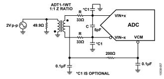
Figure 57. Differential Transformer-Coupled Configuration for Baseband Applications
