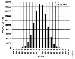
Figure 39. Input-Referred Noise Histogram, f<sub>SAMPLE</sub> = 125 MSPS, V<sub>REF</sub> = 1.3 V
