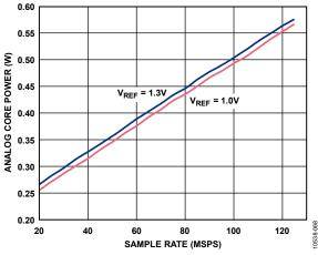
Figure 70. Analog Core Power vs.  $f_{SAMPLE}$  for  $f_{IN} = 9.7$  MHz, Four Channels
