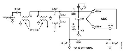
Figure 56. Differential Double Balun Input Configuration for Baseband Applications
