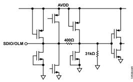
Figure 45. Equivalent SDIO/OLM Input Circuit
