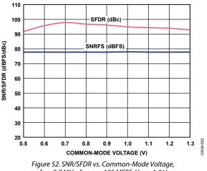
$f_{IN} = 9.7 \text{ MHz}, f_{SAMPLE} = 125 \text{ MSPS}, V_{REF} = 1.0 \text{ V}$
