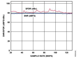
Figure 42. SNR/SFDR vs. Sample Rate,  $f_{\rm IN}$  = 64 MHz, Clock Divider = 4,  $V_{\rm REF}$  = 1.3 V
