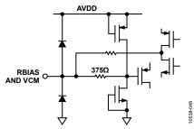
Figure 48. Equivalent RBIAS and VCM Circuit
