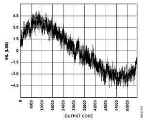
Figure 37. INL,  $f_{IN} = 9.7 \text{ MHz}$ ,  $f_{SAMPLE} = 125 \text{ MSPS}$ ,  $V_{REF} = 1.3 \text{ V}$
