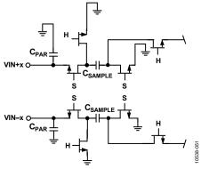
Figure 51. Switched-Capacitor Input Circuit
