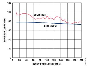
Figure 16. SNR/SFDR vs. f<sub>IN</sub>, f<sub>SAMPLE</sub> = 125 MSPS, Clock Divider = 8, V<sub>REF</sub> = 1.0 V
