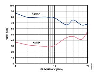
Figure 40. PSRR vs. Frequency,  $f_{SAMPLE} = 125$  MSPS,  $V_{REF} = 1.3$  V
