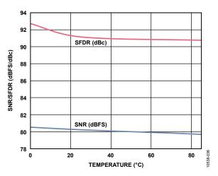
Figure 36. SNR/SFDR vs. Temperature,  $f_{IN} = 9.7 \text{ MHz}$ ,  $f_{SAMPLE} = 125 \text{ MSPS}$ ,  $V_{REF} = 1.3 \text{ V}$
