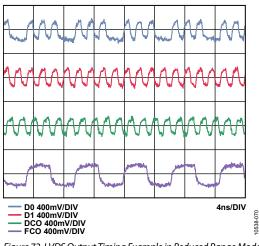
Figure 72. LVDS Output Timing Example in Reduced Range Mode
