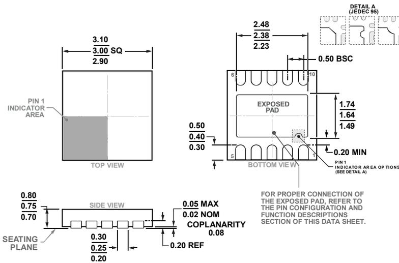
Figure 68. 10-Lead Lead Frame Chip Scale Package [LFCSP]
