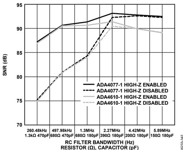
Figure 45. SNR vs. RC Filter Bandwidths for Various Precision ADC Drivers,  $f_{IN} = 1$  kHz (Turbo Mode On, High-Z Enabled/Disabled),  $V_{DD} = 1.8$  V,  $V_{IO} = 3.3$  V,  $V_{REF} = 5$  V,  $T_A = 25^\circ\text{C}$
