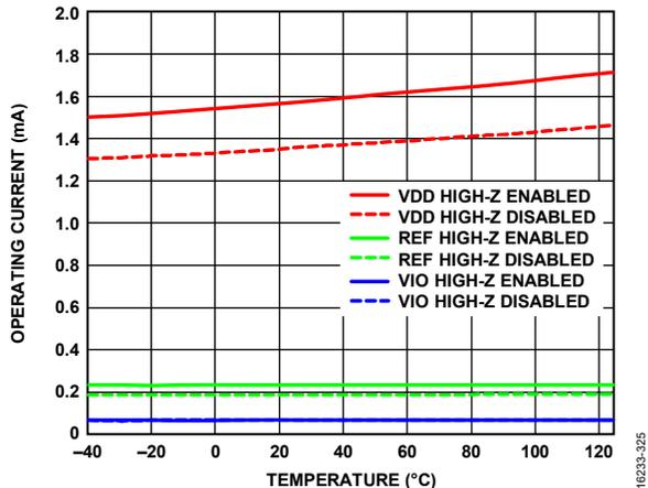
Figure 31. Operating Current vs. Temperature, AD4010, 500 kSPS
