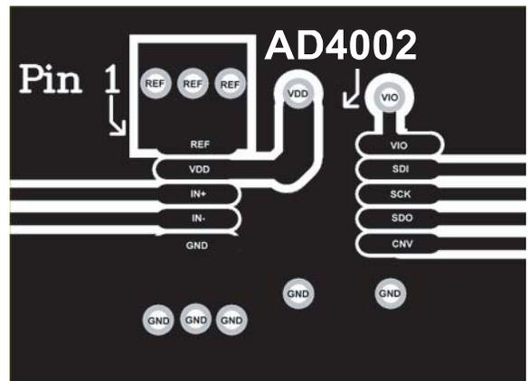
Figure 65. Example Layout of the AD4002 (Top Layer)
