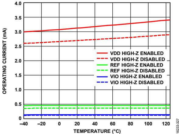
Figure 30. Operating Current vs. Temperature, AD4006, 1 MSPS
