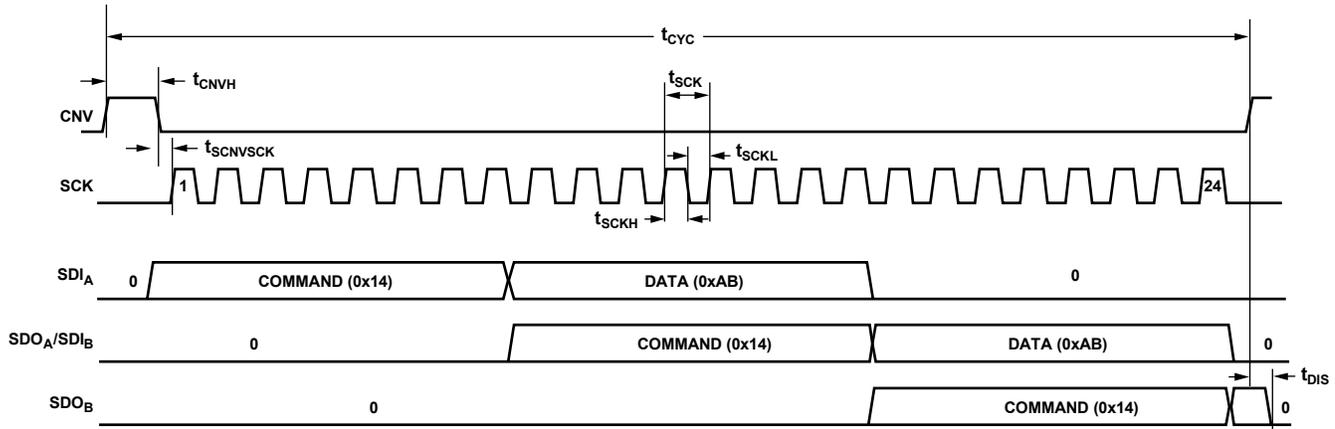
Figure 49. Register Write Timing Diagram, Daisy-Chain Mode
