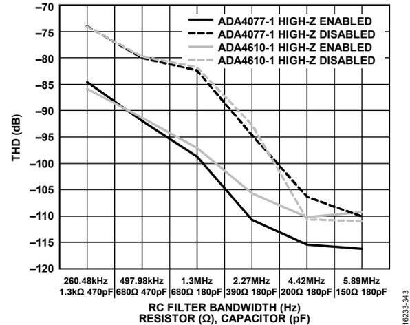
Figure 46. THD vs. RC Bandwidths for Various Precision ADC Drivers,  $f_{IN} = 1$  kHz (Turbo Mode On, High-Z Enabled/Disabled),  $V_{DD} = 1.8$  V,  $V_{IO} = 3.3$  V,  $V_{REF} = 5$  V,  $T_A = 25^\circ\text{C}$
