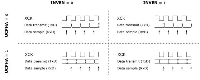
Figure 27-5. Data Transfer Timing Diagrams
