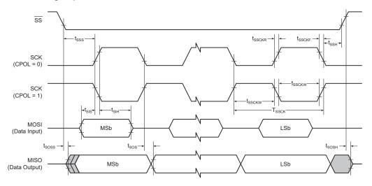
Table 36-20. SPI - Timing Specifications in Client Mode
