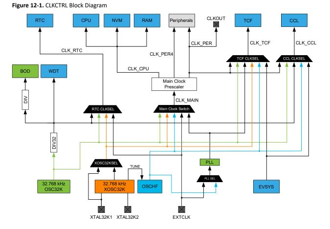
The clock system consists of the main clock and clocks derived from the main clock, as well as several asynchronous clocks:
