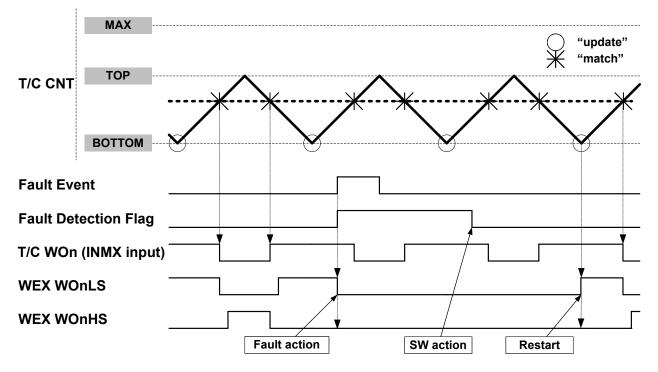
Figure 24-8. Latched Mode Fault Handling
