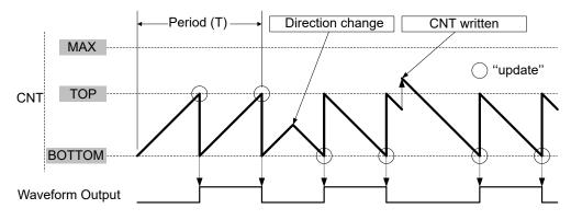
The following equation defines the waveform frequency (f<sub>FRQ</sub>):
