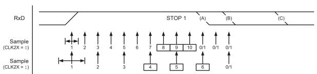
Figure 27-8. Stop Bit and Next Start Bit Sampling
