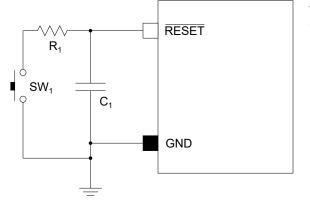
Typical values (recommended):  $C_1$ : 100 nF (filtering capacitor)  $R_1$ : 330 $\Omega$  (switch series resistance)
