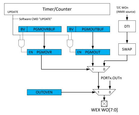
Figure 24-6. Pattern Generator Block Diagram
