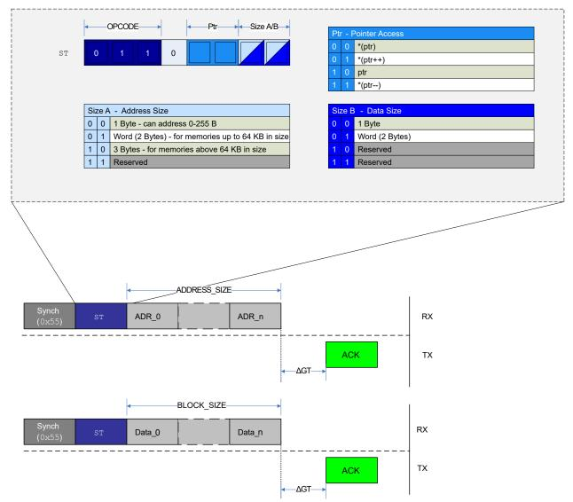
Figure 34-12 gives an example of an ST instruction to the UPDI Pointer register and the storage of regular data. A SYNCH character is sent before each instruction. In both cases, an Acknowledge (ACK) is sent back by the UPDI if the ST instruction was successful.
