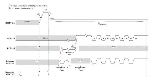
Figure 34-6. UPDI Enable Sequence by High-Voltage (HV) Programming
