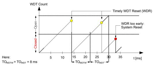
The Window mode is enabled by writing a non-zero value to the WINDOW bit field in the Control A (WDT.CTRLA) register and disabled by writing it to  $0 \times 0$ .
