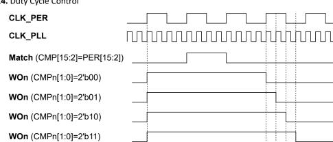
Figure 23-14. Duty Cycle Control
