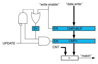
The TCEn.CMPn and TCEn.CMPnBUF registers are available as I/O registers, allowing the initialization and bypassing of the buffer register and the double-buffering function.
