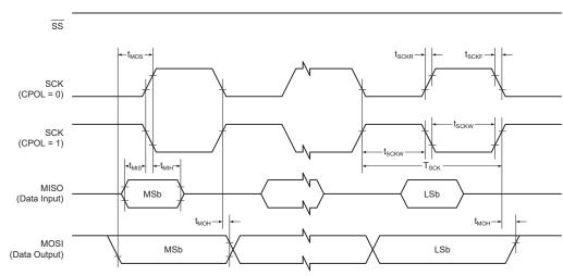
Figure 36-4. SPI - Timing Requirements in Host Mode
