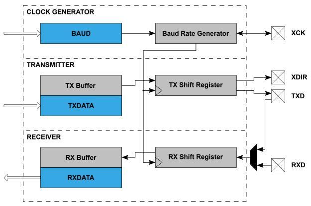
Figure 27-1. USART Block Diagram
