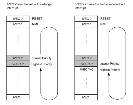
The round robin scheduling for LVL0 interrupt requests is enabled by writing a '1' to the Round Robin Priority Enable (LVL0RR) bit in the Control A (CPUINT.CTRLA) register.
