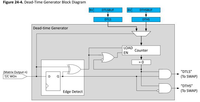
Figure 24-5 shows the 8-bit dead-time counter is decremented by one for each peripheral clock cycle until it reaches zero. A nonzero counter value will force the low and high side outputs into their OFF state.
