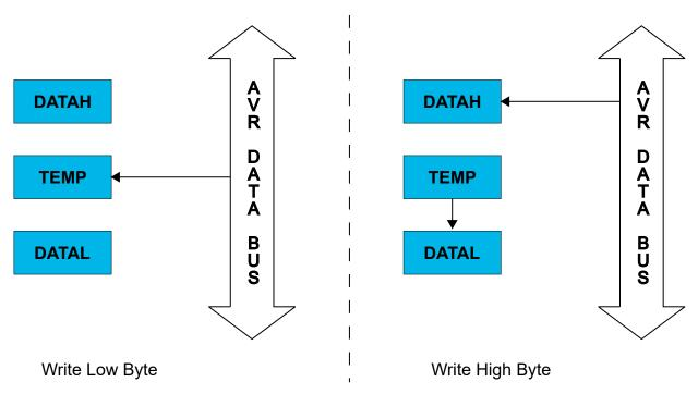
Figure 8-3. 16-Bit Register Write Operation
