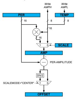
Figure 23-15. Write to Amplitude and Offset Registers
