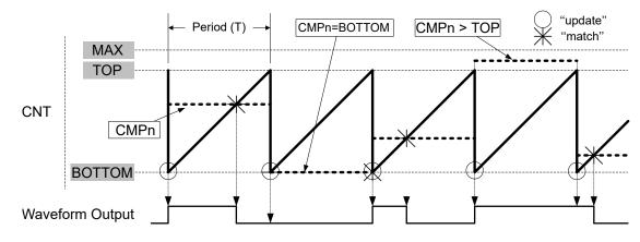
Figure 23-11. Single-Slope Pulse-Width Modulation
