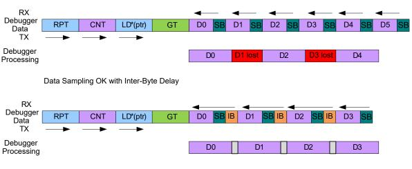
Too Fast Transmission, no Inter-Byte Delay
