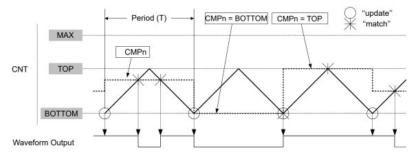
The Period (TCEn.PER) register defines the PWM resolution. The minimum resolution is two bits (TCEn.PER =  $0 \times 0003$ ), and the maximum is 16 bits (TCEn.PER = MAX).
