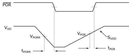
**Note:** When POR is low, the device is held in Reset.
