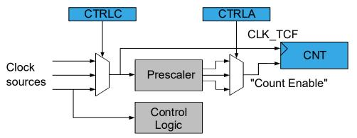
The Clock Select (CLKSEL) bit field in the Control C (TCFn.CTRLC) register selects one of the clock sources used as an input for the prescaler.
