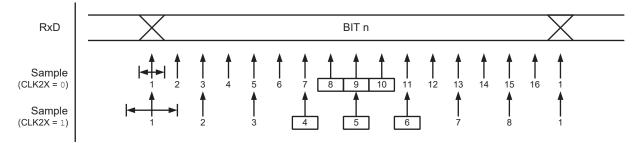
A majority voting technique is, like with clock recovery, used on the three center samples for deciding the logic level of the received bit. The process is repeated for each bit until a complete frame is received.
