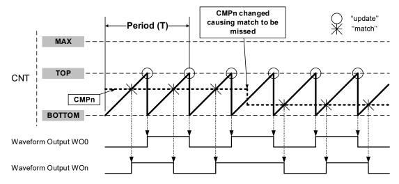
The figure below shows how the waveform can be inverted by changing the CMPn during run-time.
