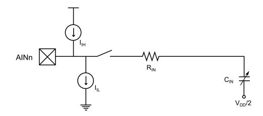
If a source with high impedance is used, the sampling time may need to be increased. The required sample time will depend on how long the source needs to charge the C<sub>IN</sub> capacitor and can be configured using the Sample Duration (SAMPDUR) bit field in the Control E (ADCn.CTRLE) register.
