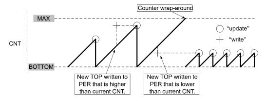
A counter wraparound can occur in any mode of operation when up-counting without buffering. This happens because the TCEn.CNT and TCEn.PER registers are continuously compared. If a new TOP value is written to TCEn.PER that is lower than current TCEn.CNT, the counter will wrap first before a compare match happens.
