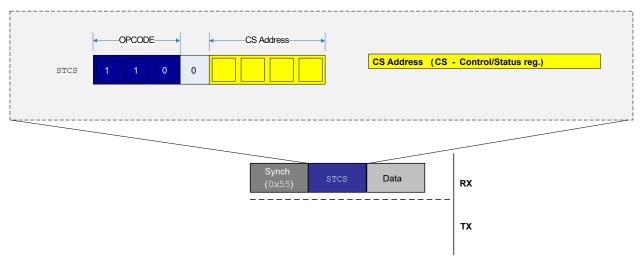
Figure 34-14 shows the data frame transmitted after the SYNCH character and the instruction frames. The STCS instruction byte can immediately be followed by the data byte. There is no response generated from the STCS instruction, as is the case for the ST and STS instructions.
