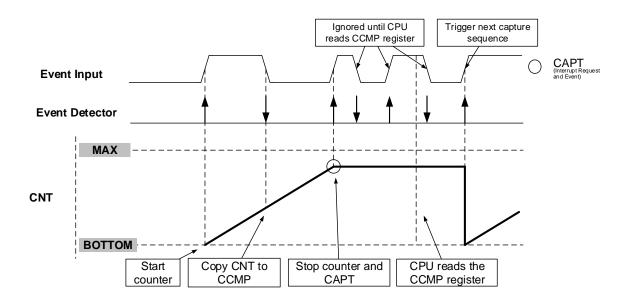
Figure 22-8. Input Capture Frequency and Pulse-Width Measurement
