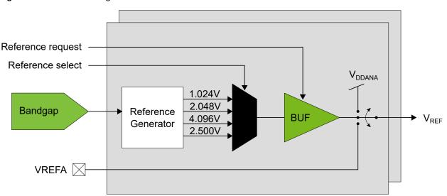
Figure 20-1. VREF Block Diagram
