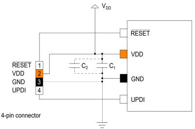
**Typical values (recommended):** C<sub>1</sub>: 100 nF (primary decoupling capacitor)
