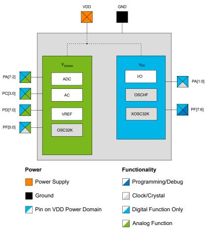
The AVR<sup>®</sup> EB Family devices have several power domains with the following power supply pins:
