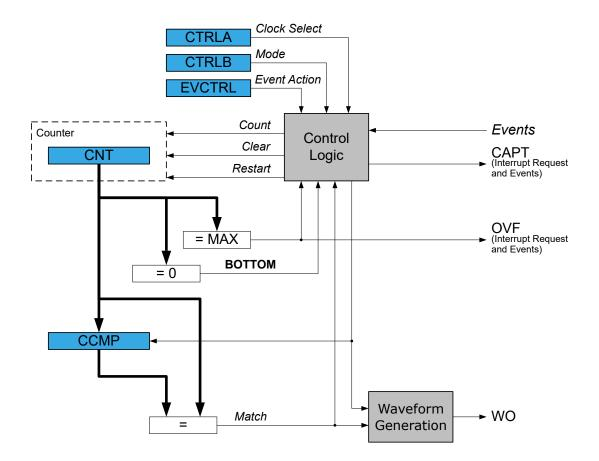
The timer/counter can be clocked from the Peripheral Clock (CLK\_PER), from a 16-bit Timer/Counter type E (CLK\_TCEn), or the Event System (EVSYS).
