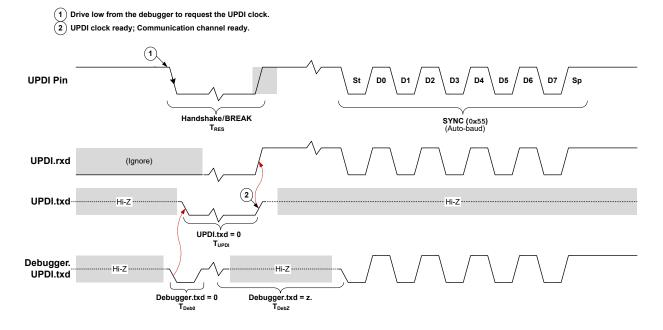
The delay given for the edge detector active drive period is a typical start-up time waiting for 256 cycles on a 32 MHz oscillator + the calibration readout. Refer to the *Electrical Characteristics* section for details on the expected start-up times.
