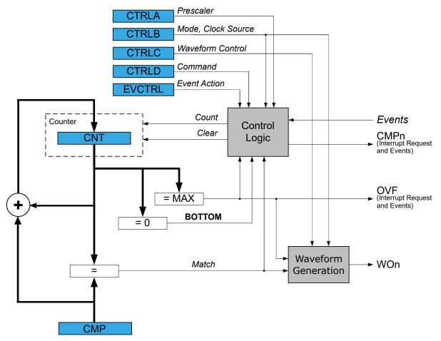
The timer/counter can be clocked from multiple clock sources, including the Peripheral Clock (CLK\_PER), internal oscillators, and Event System (EVSYS).
