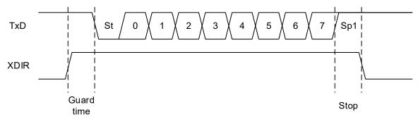
RS-485 mode is compatible with One-Wire mode. One-Wire mode enables an internal connection between the TXD pin and the USART receiver, making the TXD pin a combined TxD/RxD line.
