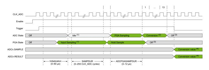
Figure 33-6. Timing Diagram - Single Conversion with PGA
