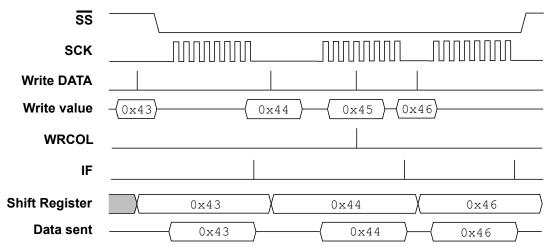
The figure above shows three transfers and one write to the DATA register while the SPI is busy with a transfer. This write will be ignored, and the Write Collision (WRCOL) flag in SPIn.INTFLAGS is set.
