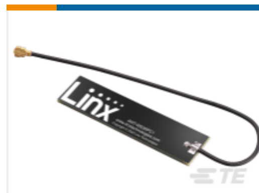
TE Part #ANT-W63RPC1-100 Antenna WIFI6 2.4/5/6 GHz RPC Cut 100
