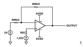
Figure 7. DC Voltage Source Input Test Circuit, Shunt installed at P4 and P4
