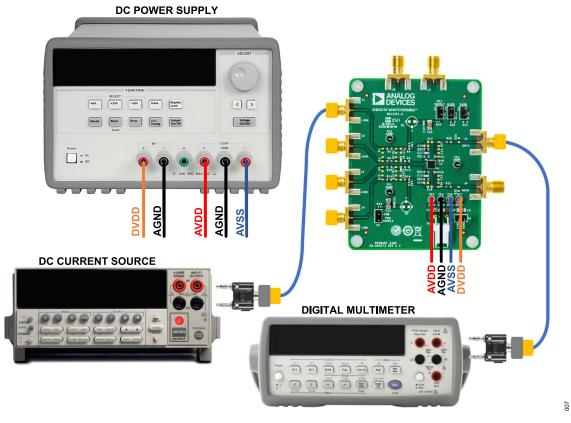
Figure 5. EVAL-ADA4351-2EBZ Full Setup for Current Source Input
