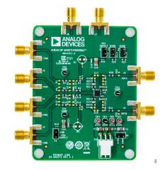
Figure 1. EVAL-ADA4351-2EBZ Photograph (Top View)
