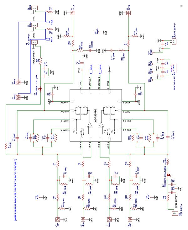
Figure 8. EVAL-ADA4351-2EBZ Evaluation Board Schematic
