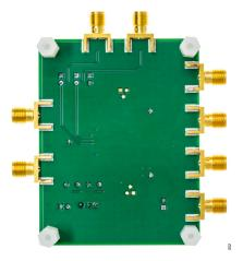
Figure 2. EVAL-ADA4351-2EBZ Photograph (Bottom View)
