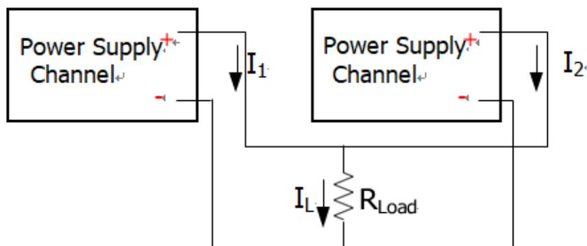
When two insulated channels are connected in parallel:  $I_L = I_1 + I_2$
