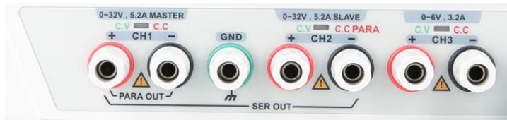
1. Each channel can be used as an independent channel.
