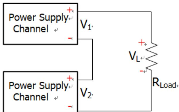
When two insulated channels are connected in series:  $V_L = V_1 + V_2$
