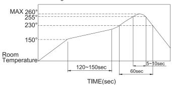
The condition mentioned above is the temperature on the Cu foil of the PCB surface.
