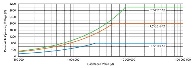
The permissible operating voltage  $\textit{U}_{max.}$  equals the rated voltage. For ambient temperatures above 70 °C power derating must be considered
