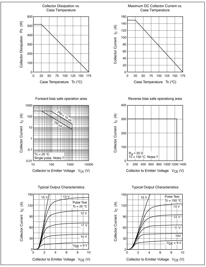
Notes: 7. Designed target value on Renesas measurement condition. (Not tested) Renesas recommends that operating conditions are designed according to a document "Power MOS FET • IGBT Attention of Handling Semiconductor Devices".
