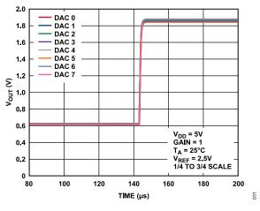
Figure 29. Full-Scale Settling Time
