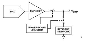
Figure 46. Output Stage During Power-Down
