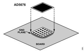
Figure 51. Pad Connection to Board
