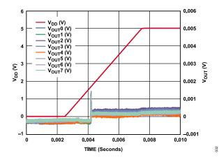
Figure 30. Power-On Reset to 0 V and Midscale
