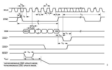
Figure 2. Serial Write Operation
