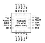
NOTES 1. NIC = NOT INTERNALLY CONNECTED. 2. EXPOSED PAD. THE EXPOSED PAD MUST BE TIED TO GND. §
