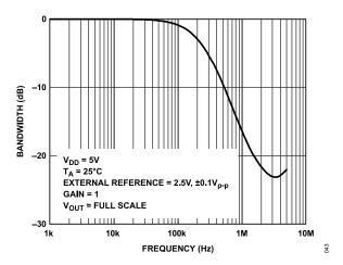
Figure 41. Multiplying Bandwidth, External Reference
