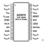
Figure 6. 20-Lead TSSOP Pin Configuration
