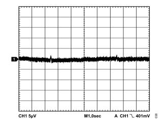
Figure 35. 0.1 Hz to 10 Hz Output Noise
