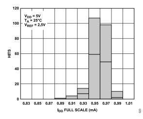
Figure 21. I<sub>DD</sub> Histogram with External Reference
