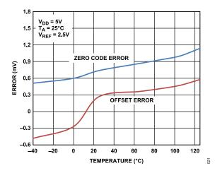
Figure 19. Zero Code Error and Offset Error vs. Temperature
