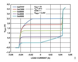
Figure 24. Source and Sink Capability at 3 V
