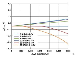
Figure 22. Headroom/Footroom ( $\Delta V_{OUT}$ ) vs. Load Current
