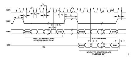
Figure 5. Readback Timing Diagram
