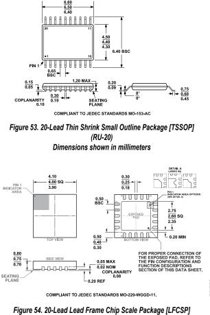
4 mm × 4 mm Body and 0.75 mm Package Height (CP-20-8) Dimensions shown in millimeters
