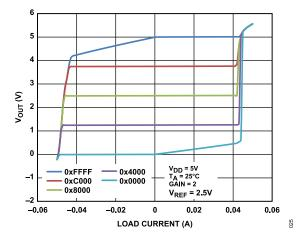
Figure 23. Source and Sink Capability at 5 V
