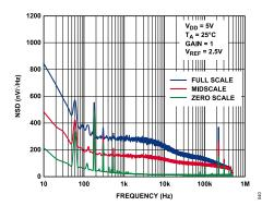
Figure 36. Noise Spectral Density (NSD)
