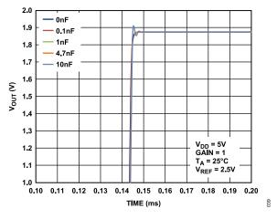
Figure 38. Settling Time for Various Capacitive Loads
