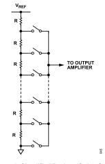
Figure 43. Simplified Resistor String Structure
