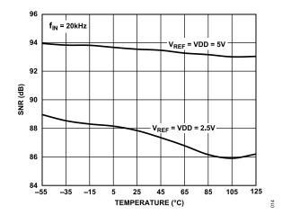
Figure 16. SNR vs. Temperature
