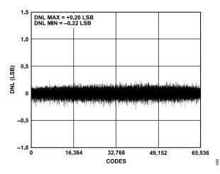
Figure 11. Differential Nonlinearity vs. Code,  $V_{REF} = VDD = 5 V$
