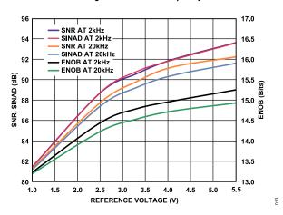
Figure 15. SNR, SINAD, and Effective Number of Bits (ENOB) vs. Reference Voltage
