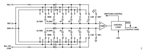
Figure 26. ADC Simplified Schematic
