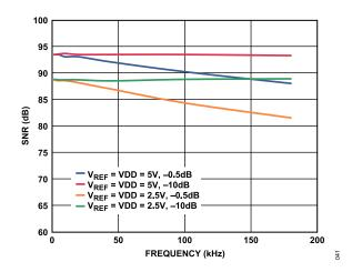
Figure 14. SNR vs. Frequency
