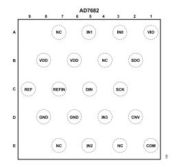
Figure 6. AD7682 WLCSP Pin Configuration
