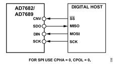
Figure 42. Connection Diagram for the AD7682/AD7689 Without a Busy Indicator
