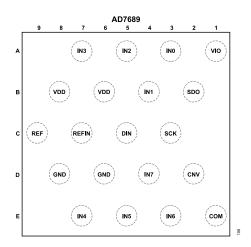
Figure 7. AD7689 WLCSP Pin Configuration
