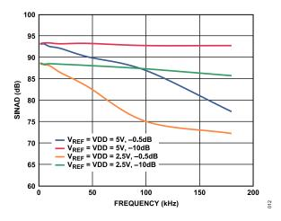
Figure 17. SINAD vs. Frequency
