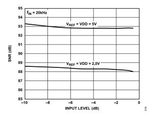
Figure 21. SNR vs. Input Level
