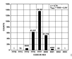
Figure 12. Histogram of a DC Input at Code Center
