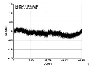
Figure 8. Integral Nonlinearity vs. Code,  $V_{REF} = VDD = 5 V$
