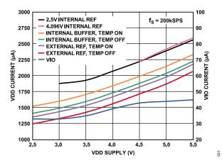
Figure 23. Operating Currents vs. Supply
