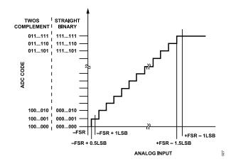
Figure 27. ADC Ideal Transfer Function
