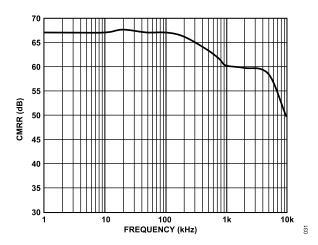
Figure 31. Analog Input CMRR vs. Frequency
