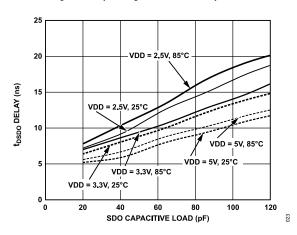
Figure 25. t<sub>DSDO</sub> Delay vs. SDO Capacitance Load and Supply
