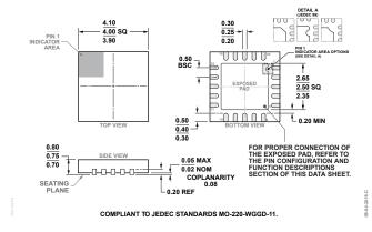
Figure 46. 20-Lead Lead Frame Chip Scale Package [LFCSP] 4 mm × 4 mm Body and 0.75 mm Package Height (CP-20-10)
