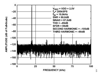
Figure 13. 20 kHz FFT,  $V_{REF} = VDD = 2.5 V$
