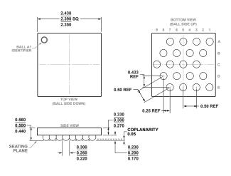
Figure 48. 20-Ball Wafer Level Chip Scale Package [WLCSP] (CB-20-12) Dimensions shown in millimeters
