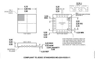
Figure 47. 20-Lead Lead Frame Chip Scale Package [LFCSP] 4 mm × 4 mm Body and 0.85 mm Package Height (CP-20-22)
