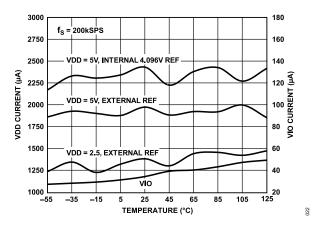
Figure 24. Operating Currents vs. Temperature
