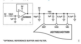
Figure 38. Example of an Application Circuit
