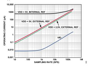
Figure 37. Operating Currents vs. Sampling Rate
