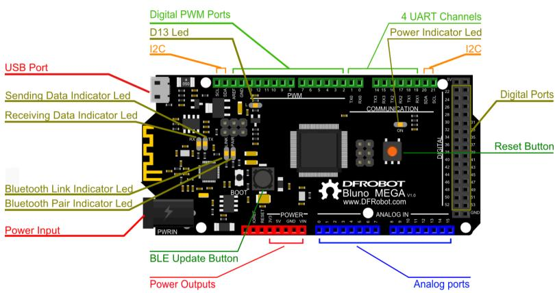
The figure above shows Bluno Mega2560 controller with all the ports, which includes:
