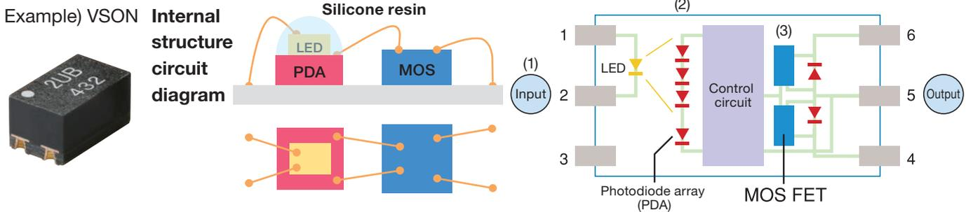
1. The LED lights up when the current flows to the input side.
