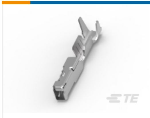
TE Part #2098762-4 Contact,female0.64, 22 AWG, CuNiSi, Sn
