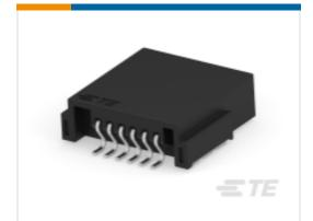
TE Part #2311714-1 6POS,TAB0.5X0.4,HDR ASSY,90DEG, COD A
