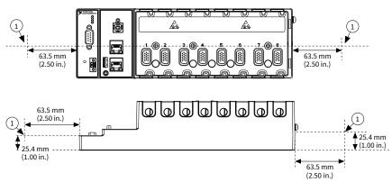
1. Location for measuring the ambient temperature
