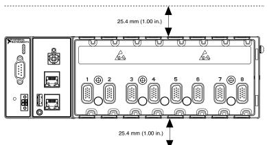
Allow the appropriate space in front of C Series modules for cabling clearance, as shown in the following figure. The different connector types on C Series modules require different cabling clearances. For a complete list of cabling clearances for C Series modules, visit <u>ni.com/info</u> and enter the Info Code crioconn.
