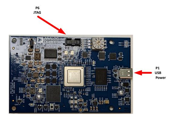
Figure 3-8: Connector Locations Top View
