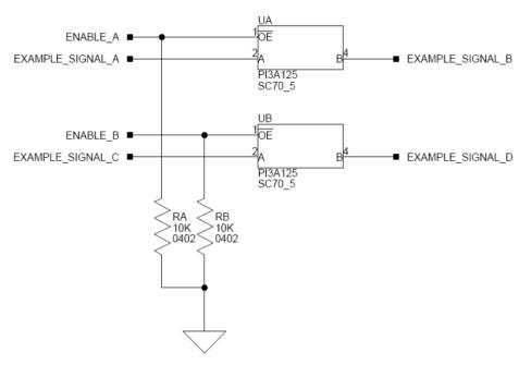
Figure 3-2: Example of Individual FET Switches
