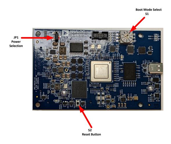
Figure 2-2: Default Hardware Setup
