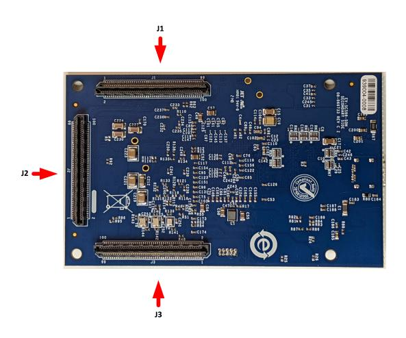
Figure 3-9: Connector Locations Bottom View
