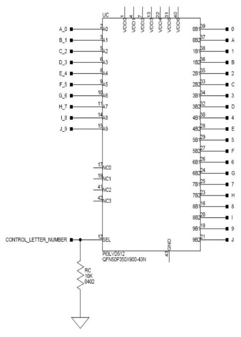
Figure 3-4: Example of a Bus Switch
