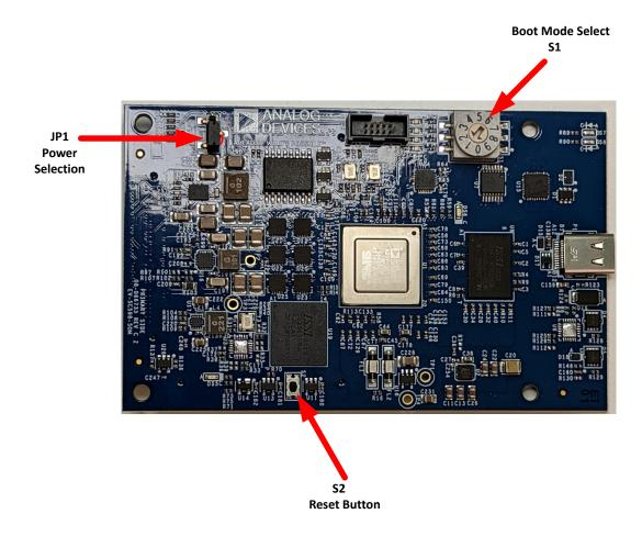
Figure 3-6: Switch/Jumper Locations
