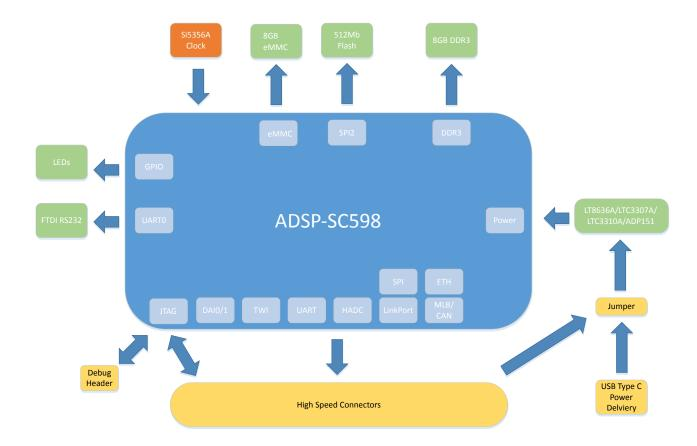
Figure 3-1: Block Diagram
