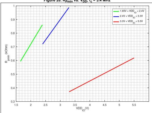
Figure 28.  $R_{Pmin}$  vs.  $V_{DD}$ ,  $f_c$  = 3.4 MHz
