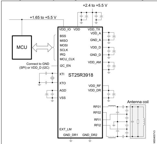
Figure 2. Minimum system configuration - Differential antenna driving
