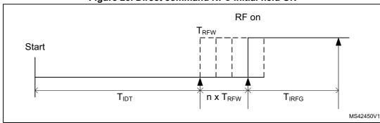
Figure 25. Direct command NFC initial field ON
