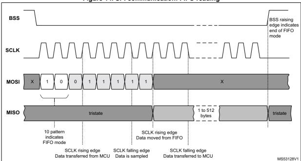
Figure 14. SPI communication: FIFO reading
