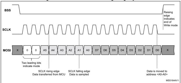
Figure 10. SPI communication: writing a single byte
