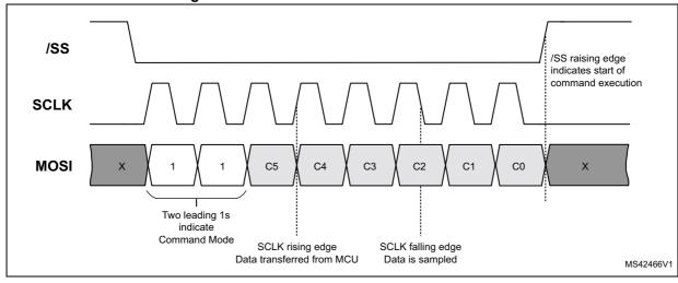
Figure 15. SPI communication: direct command
