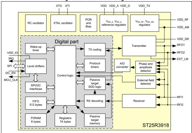
Figure 3. ST25R3918 block diagram
