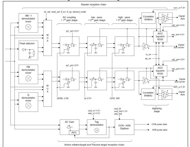
Figure 5. Receiver block diagram
