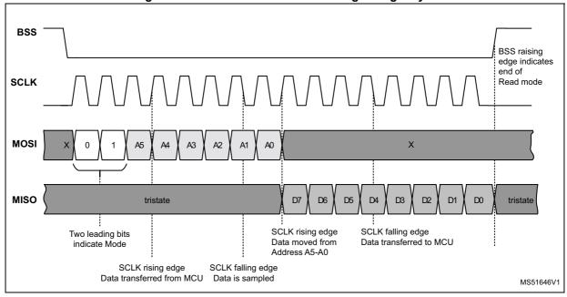
Figure 12. SPI communication: reading a single byte
