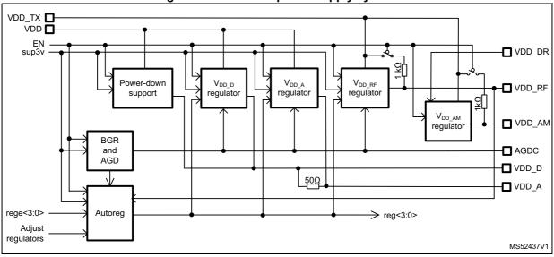
Figure 8. ST25R3918 power supply system
