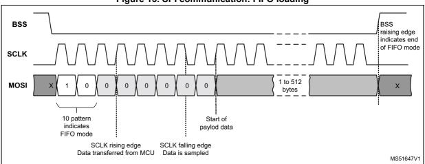
Figure 13. SPI communication: FIFO loading
