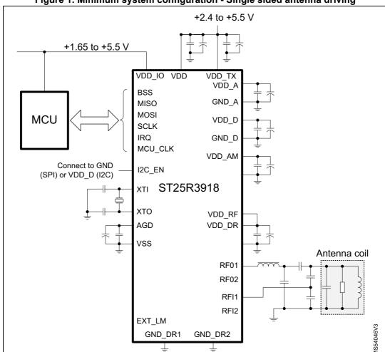
Figure 1. Minimum system configuration - Single sided antenna driving
