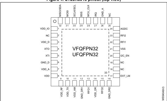
Figure 4. ST25R3918 pinout (top view)
