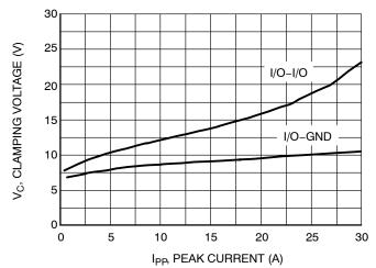
Figure 3. Clamping Voltage, 8/20 μs Waveform
