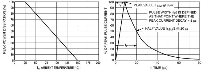
Figure 1. Pulse Derating Curve
