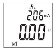
The leads are also compensated for resistance measurements.
