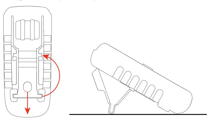
The stand can also be used to hook the instrument on a door.
