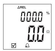
At each new measurement, the instrument indicates the difference between the new reading and the reference measurement, along with the difference in %.
