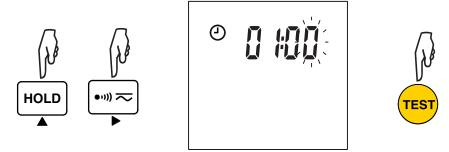
The duration can be programmed from 00:10 to 39:59 (from 10 seconds to 40 minutes).
