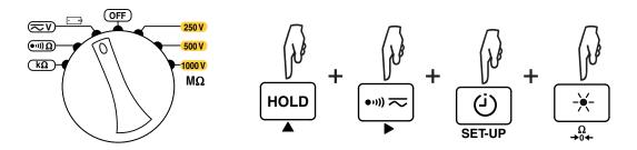
At each step, press the **TEST** key. The instrument performs the adjustment and displays the result (**PASS** or **FAIL**) Press the ▶ key to go to the next step or ▲ to return to the previous step.
