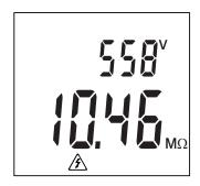
Press the **TEST** button and keep it pressed until the measurement is stable. The symbol indicates that the instrument is generating a hazardous voltage.
