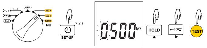
Use the ▲ key to set the digit and the ▶ key to go to the next digit. When all 4 digits have been set, choose the unit. Confirm by pressing the **TEST** button.
