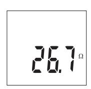
To make sure that there is no voltage, you can make a voltage measurement before the continuity measurement. Otherwise, the instrument will report the presence of a voltage if there is one.
