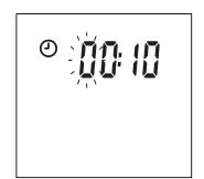
■ Use the ▲ key to set the digit and the ▶ key to go to the next digit. Confirm by pressing the **TEST** button.
