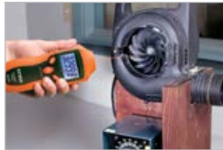
Measures the speed (RPM) of rotating objects and counts (revolution) of moving objects.
