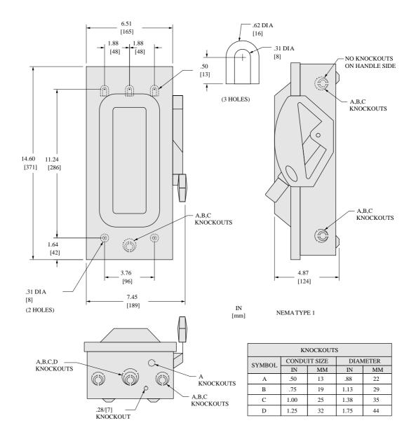
ALL DIMENSIONS ARE APPROXIMATE. WHEN MOUNTING THESE SWITCHES, ALLOW 3.00/[76] MINIMUM CLEARANCE BETWEEN ENCLOSURES FOR OPENING OF SIDE HINGED DOOR. REFER TO TECHNICAL DRAWINGS AND DOCUMENTS.
