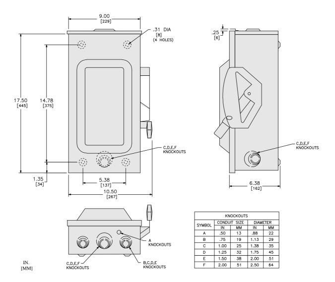
WHEN MOUNTING, ALLOW 4.00/[102] MIN. CLEARANCE BETWEEN ENCLOSURES FOR OPENING OF SIDE HINGED DOOR.
