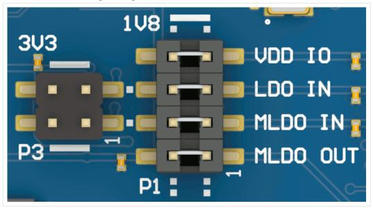
For the use-case case *Maximum RF output power and optimum system power* you have to use the following configuration:
