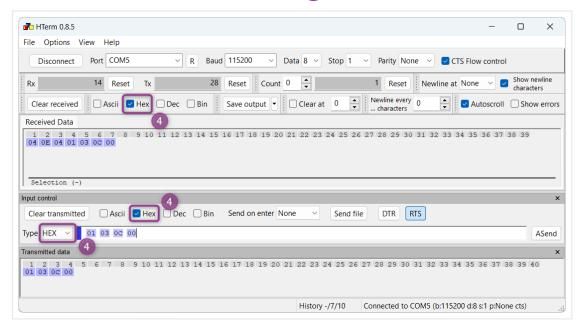
5. Enter the HCl Reset command in binary form as 01 03 0c 00 and press
