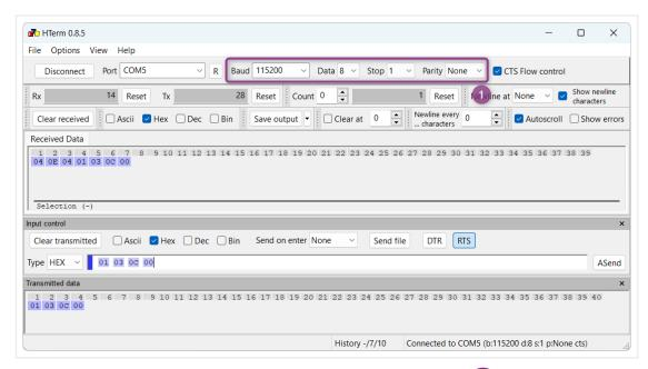
2. Open the serial port the evaluation board is connected to 2
