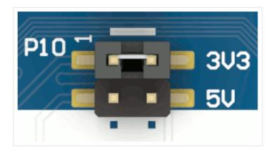
By default only the jumper that connects the 3.3 V support from the host controller board to the evaluation board is populated which is completely sufficient.
