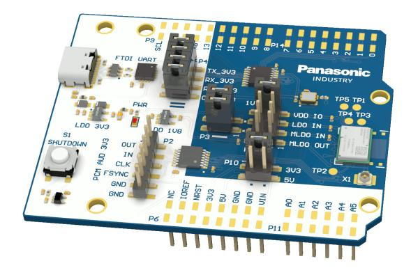
The evaluation board features a PAN1316C dual-mode Bluetooth® module which is based on the Texas Instruments CC2564C single-chip controller.
