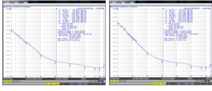
F=156.2500MHz | V<sub>dd</sub>=3.3V | LVDS RMS Phase Jitter = 88 fsec
