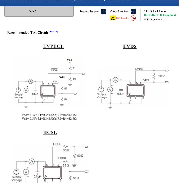
Note 11: Recommended test circuit images are representative of when the OE Function is located on Pin 1; when the OE Function is located on Pin 2, then Pin 1=No Connect & Pin 2=OE or No Connect.
