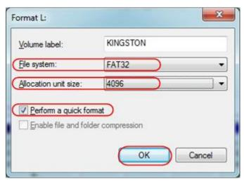
Figure 4-4: Formatting the USB disk setting
