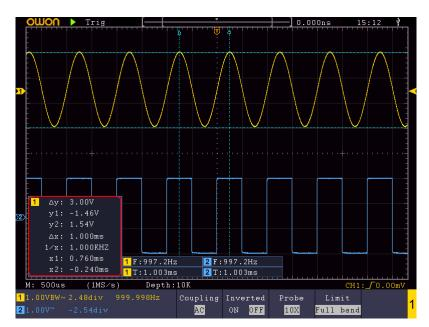
Figure 4-16 Time&Voltage Cursor Measurement
