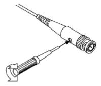
Figure 3-8 Adjust Probe
