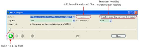
Figure 4-12: Play back waveform by software
