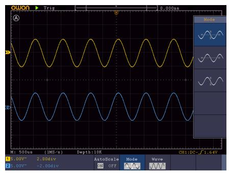
Figure 4-17 Autoscale Horizontal-Vertical multi-period waveforms
