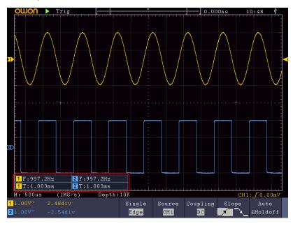
Figure 4-13 Automatic measurement
