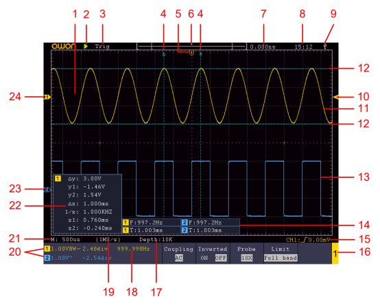
Figure 3-5 Illustrative Drawing of Display Interfaces
