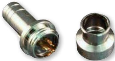
880-025P in-line plugs with solder cup contacts feature thread-on rear adapter allowing access to contacts. Install cable shield braid directly to connector with Band-Master Micro band. Three contact sizes are available with current ratings of 5A, 3A and 1A. Aluminum or stainless steel housings and thermoplastic insulators. Ultraminiature SuperFly® connectors are ideal where ruggedness and field reparability is required.
