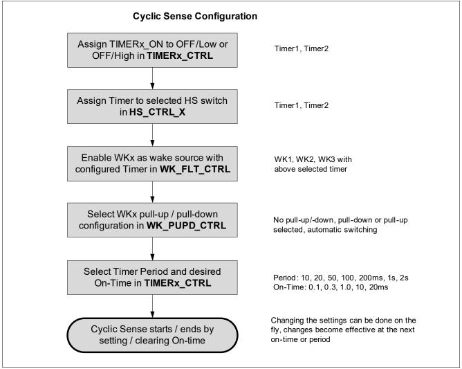
Figure 6Cyclic Sense: Configuration and Sequence
