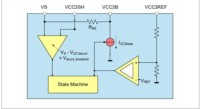
Figure 17 Functional Block Diagram
