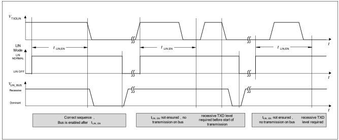
Figure 34 LIN Transceiver Enabling Sequence
