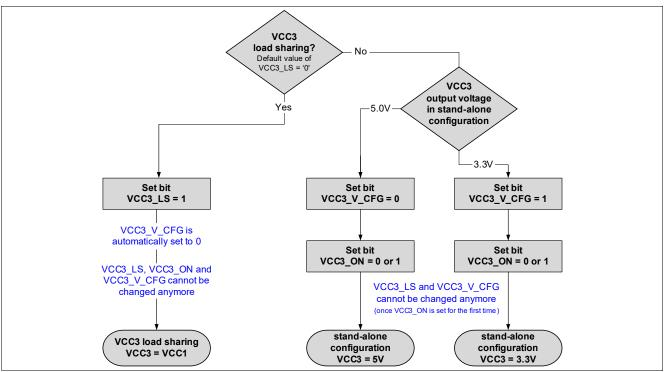
Figure 18 Selecting the Configuration of the VCC3 Regulator
