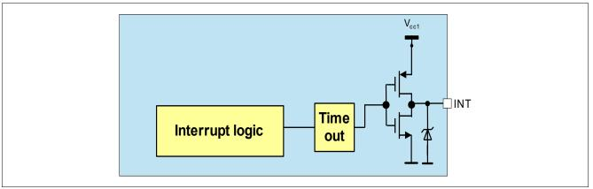
Figure 42 Interrupt Block Diagram
