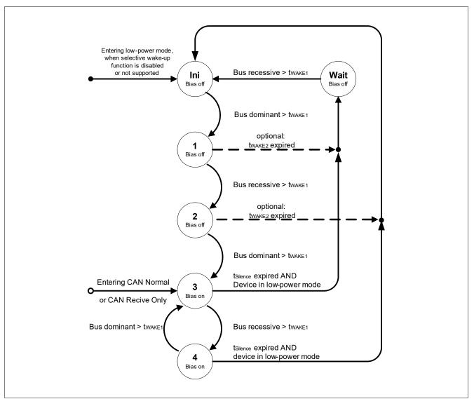
Figure 29 WUP detection following the definition in ISO 11898-2:2016
