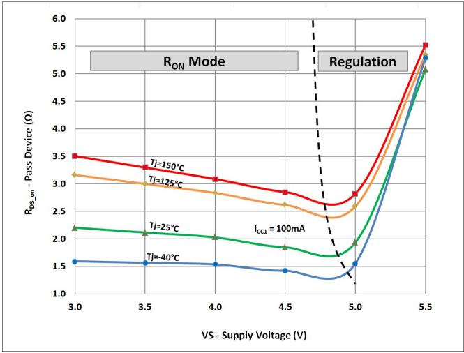
Figure 12 Typical on-resistance of VCC1 pass device during low drop operation for  $I_{CC1}$  = 100mA
