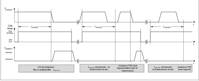
Figure 28 CAN Transceiver Enabling Sequence
