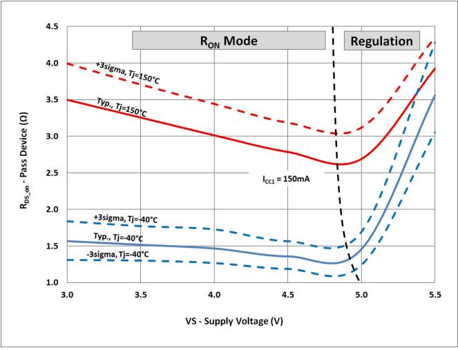
Figure 13 On-resistance range of VCC1 pass device during low drop operation for  $I_{CC1}$  = 150mA
