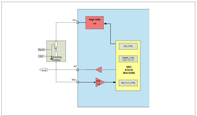
Figure 5 Cyclic Sense Working Principle
