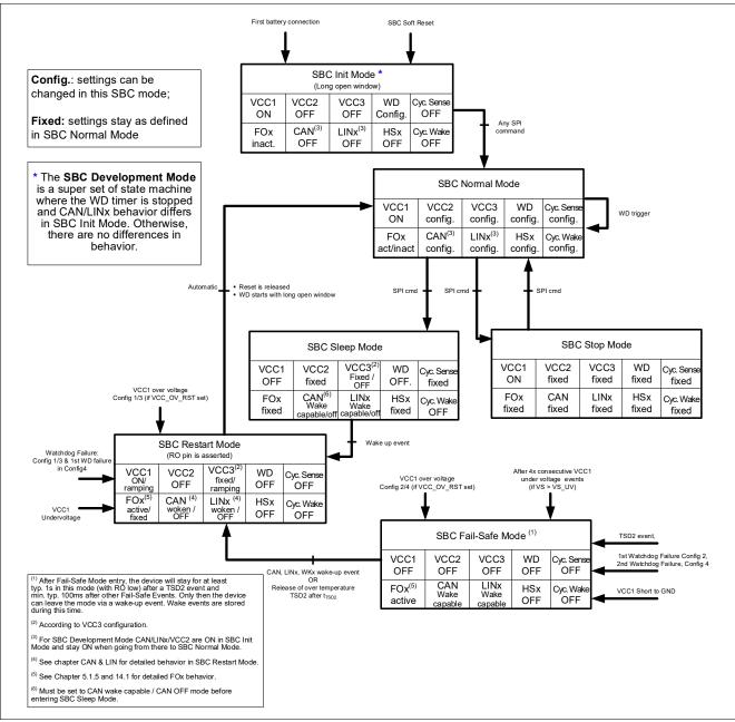
Figure 3 State Diagram showing the SBC Operating Modes
