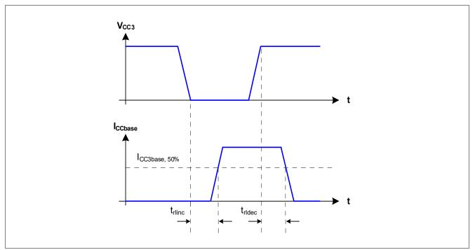
Figure 21 Regulator Reaction Time
