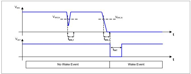
Figure 39 Wake-up Filter Timing for Static Sense
