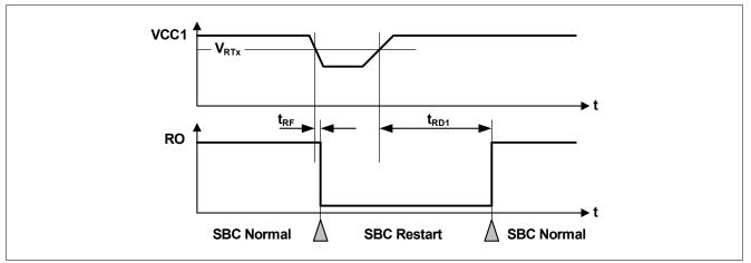
Figure 52 VCC1 Undervoltage Timing Diagram
