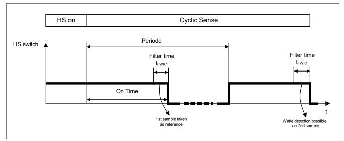
Figure 7 Wake Input Timing
