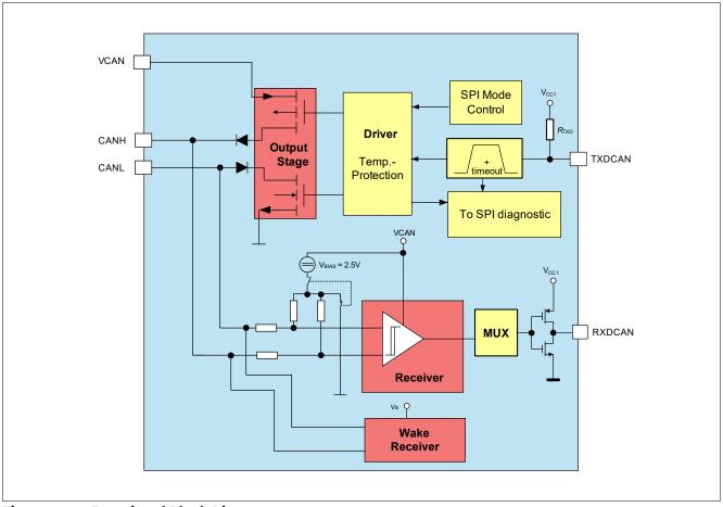
Figure 25 Functional Block Diagram
