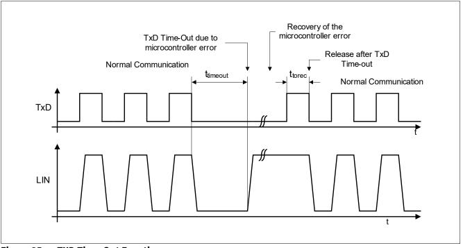
Figure 35 TXD Time-Out Function
