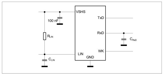
Figure 36 Simplified Test Circuit for Dynamic Characteristics
