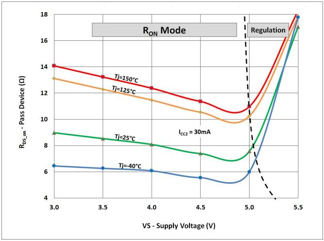
Figure 15Typical on-resistance of VCC2 pass device during low drop operation for  $I_{CC2}$  = 30mA
