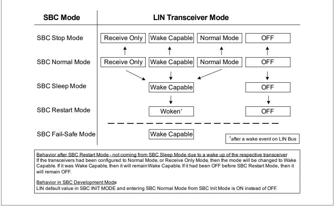
Figure 33 LIN Mode Control Diagram
