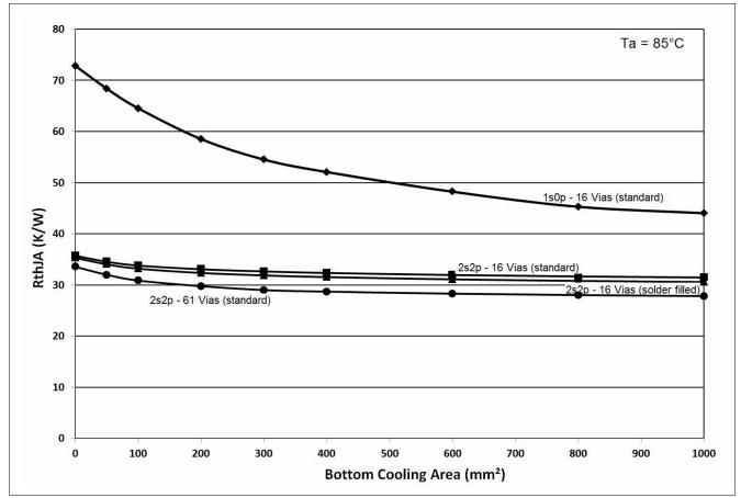
Figure 62Thermal Resistance  $(R_{th_{JA}})$  vs. Cooling Area
