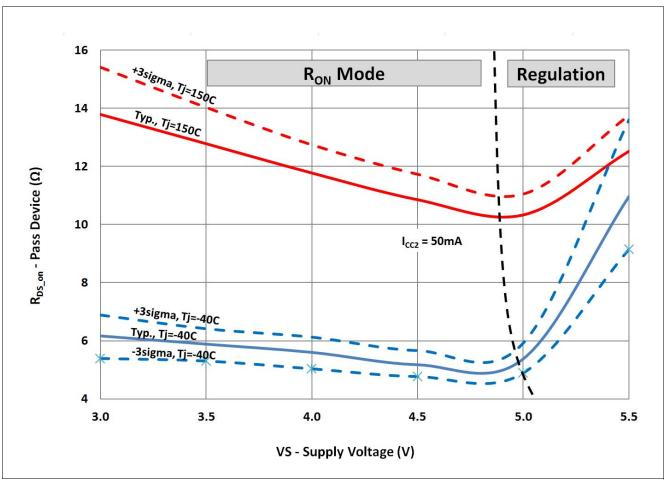
Figure 16 On-resistance range of VCC2 pass device during low drop operation for I<sub>cc2</sub> = 50mA
