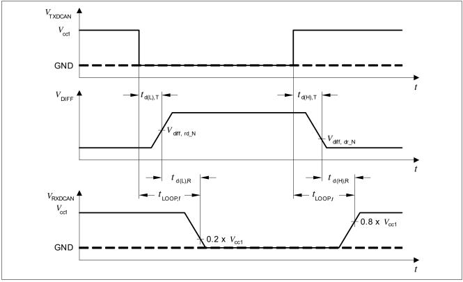
Figure 30 Timing Diagrams for Dynamic Characteristics
