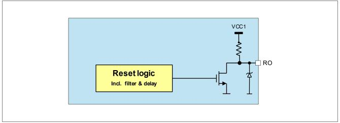
Figure 46 Reset Block Diagram
