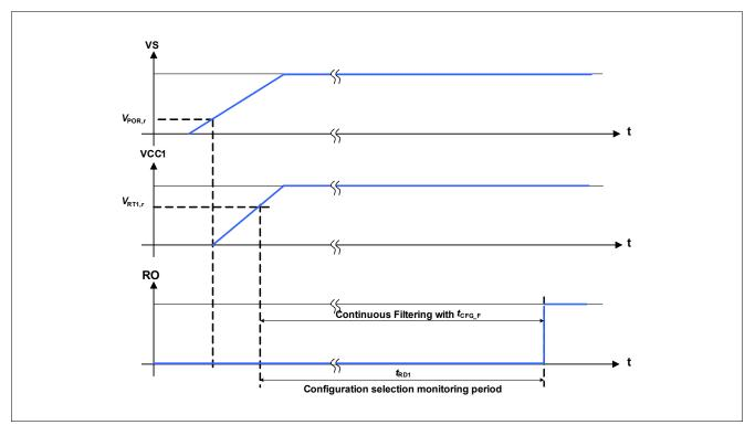
Figure 4 Hardware Configuration Selection Timing Diagram
