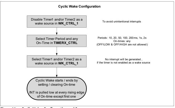
Figure 10 Cyclic Wake: Configuration and Sequence
