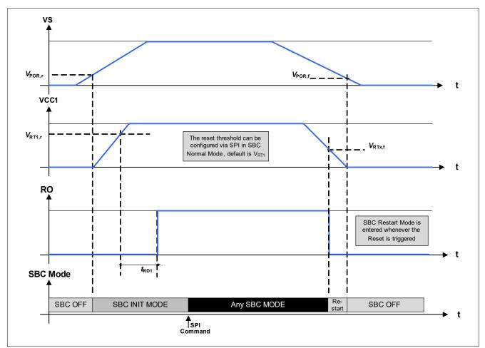
Figure 51 Ramp up / down example of Supply Voltage
