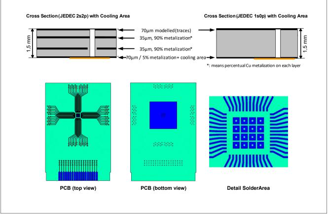
Figure 63 Board Setup
