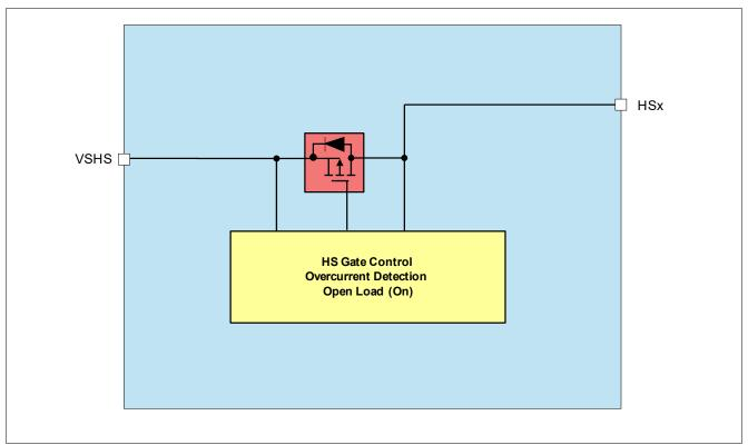
Figure 24 High-Side Module Block Diagram
