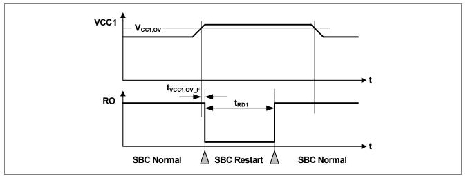
Figure 53 VCC1 Overvoltage Timing Diagram
