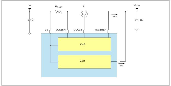
Figure 20 VCC3 in Load Sharing Configuration
