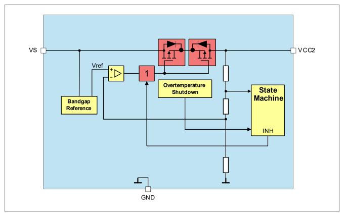
Figure 14 Module Block Diagram
