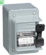
Switch, manual, 30A, 3 pole, 10 HP at 575 VAC, three phase, toggle operated, no indicator, NEMA 4, one conduit opening
