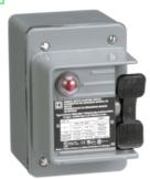
Switch, manual, 30A, 2 pole, 3 HP at 575 VAC, single phase, toggle operated, red 115 VAC indicator, NEMA 4, one conduit
