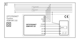
OT 4DIM NFC G3 Wiring Diagram I
