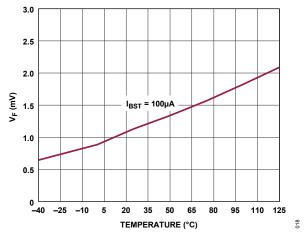
Figure 18. Bootstrap Switch Voltage vs. Temperature
