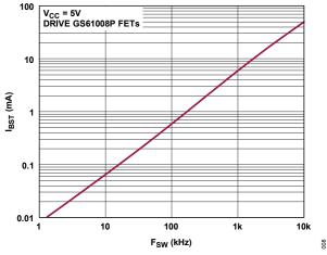
Figure 8. BST Operating Current vs. Switching Frequency
