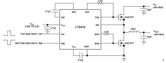
Figure 1. Highly Efficient GaN-Based Switching DC-DC Converter
