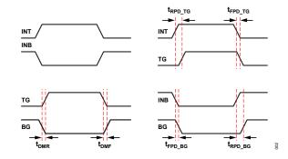
Figure 2. Timing Definitions of Propagation Delay and Delay Matching
