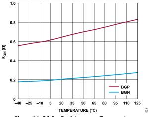
Figure 21. BG On-Resistance vs. Temperature
