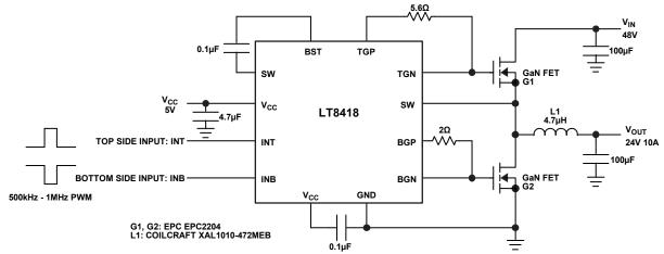
Figure 24. 48V Input, 24V and 10A Output, 500kHz to 1MHz Buck Converter
