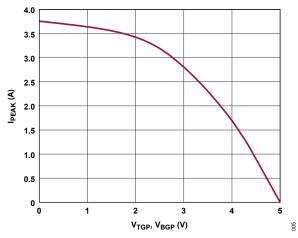
Figure 5. Peak Source Current vs. Driver Ouput Voltage
