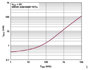
Figure 7. V<sub>cc</sub> Operating Current vs. Switching Frequency
