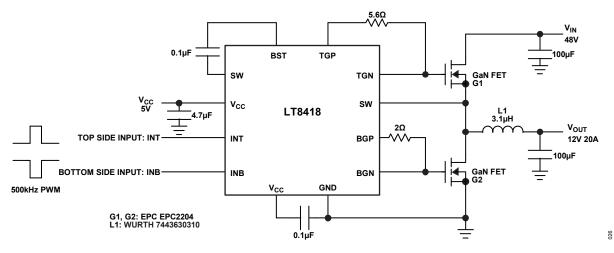
*Figure 26. 48V Input, 12V 20A Output, 500kHz Buck Converter*
