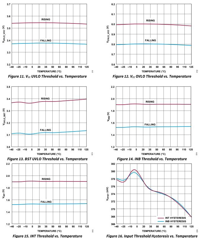
Figure 16. Input Threshold Hysteresis vs. Temperature
