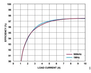
Figure 25. Efficiency vs. Load Current (with Forced Air)
