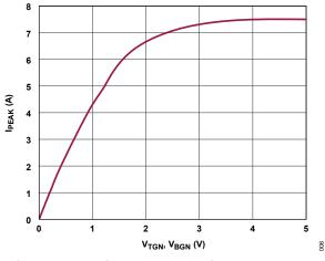
Figure 6. Peak Sink Current vs. Driver Ouput Voltage
