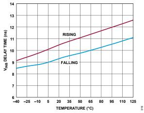
Figure 19. INB Propagation Delay vs. Temperature
