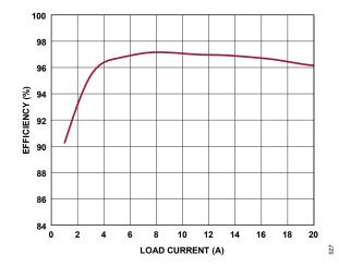
Figure 27. Efficiency vs. Load Current (with Heat Sink)
