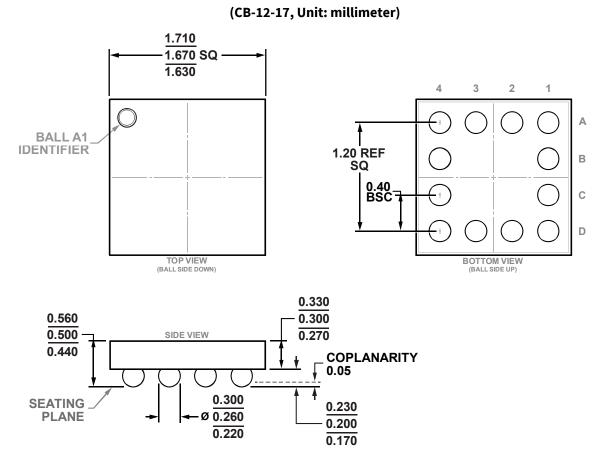
12-Ball Wafer Level Chip Scale Package (WLCSP)
