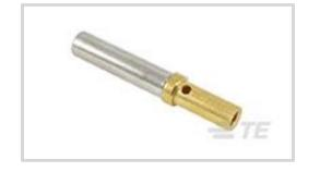
Terminal Type: Socket Mating Pin Diameter: 1.59 mm [.063 in ] Terminal Transmits: 0 – 24 A (Low Power) Wire Size: .5 – 1.3 mm<sup>2</sup>
