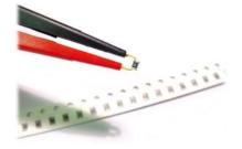
The Atlas LCR is designed to test discrete, unconnected components. Testing of components "in-circuit" will result in unpredictable measurements.
