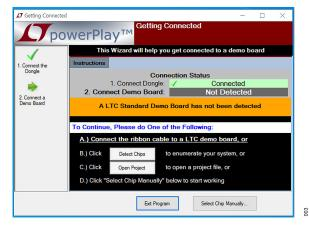
Figure 3. LTpowerPlay—Getting Connected Window
