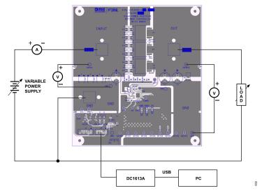
Figure 2. Basic EVAL-LTC4286-A1Z Connection Diagram
