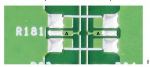
Figure 9. Sense Resistor—Kelvin Footprint
