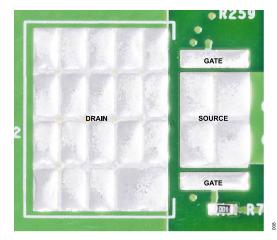
Figure 8. Multipackage N-Channel MOSFET Footprint
