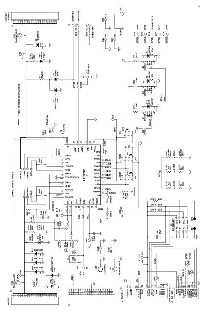
Figure 11. EVAL-LTC4286-A1Z Schematic Part 1
