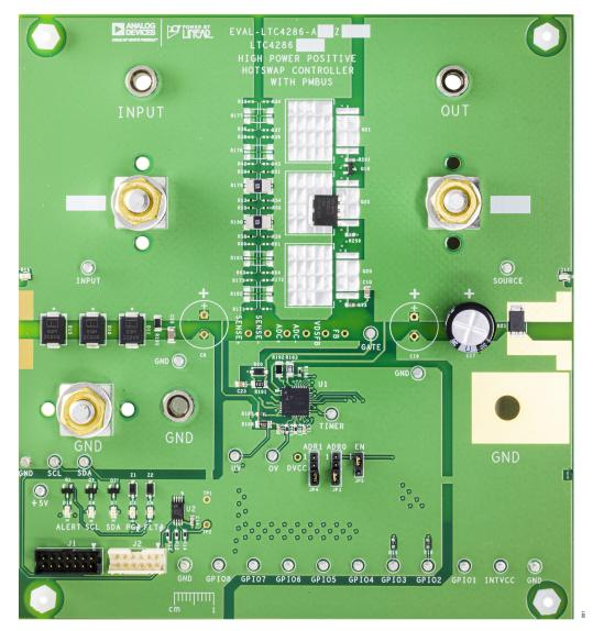
Figure 1. Evaluation Board Layout
