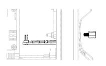
Holding the GPIB board at the edges, place the board so that the GPIB connector is protruding through the rear panel and fasten using the two M4 hex screws provided (Torque 40cNm).
