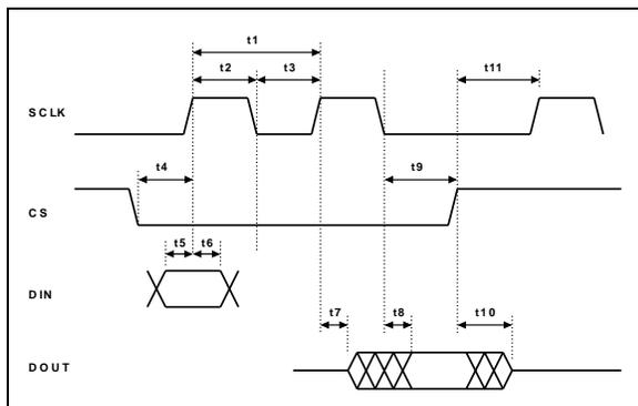
Figure 8. SPI Timing.
