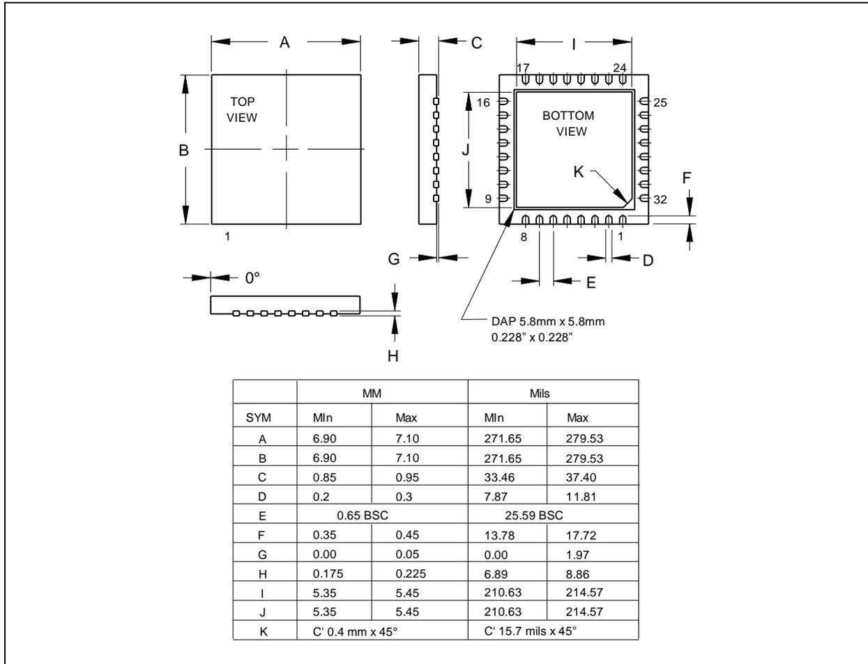
Figure 17. 7 x 7mm QFN32 Package Dimensions.
