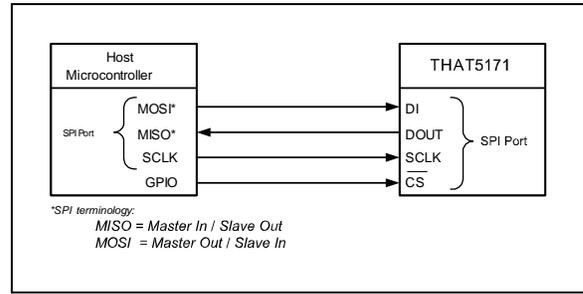
Figure 13. Single 5171 connected to a host microcontroller.
