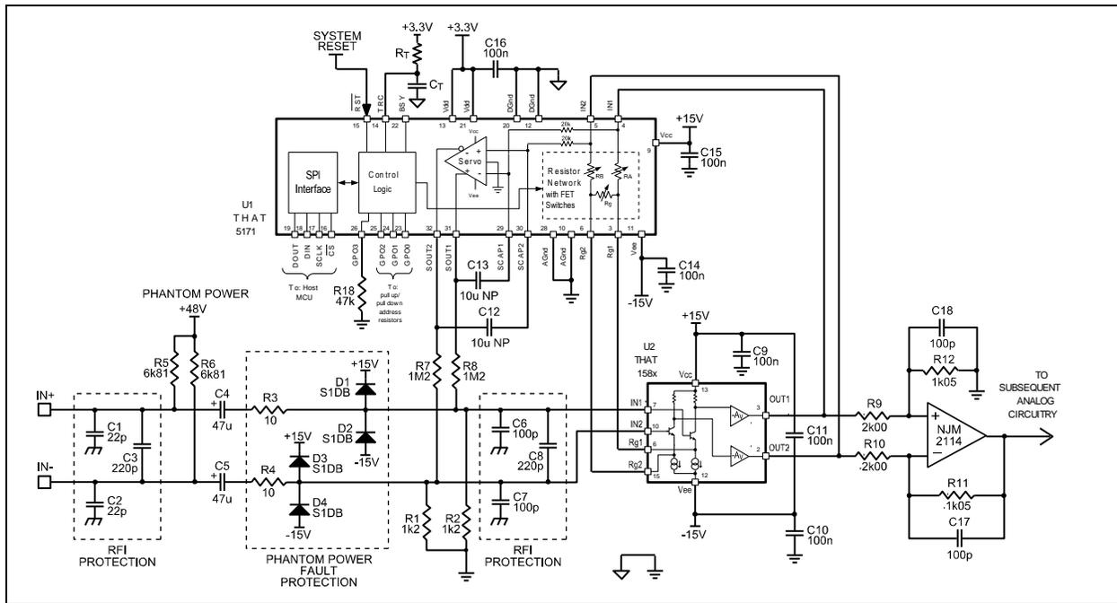
Figure 5. 5171/158x typical application with single-ended output.
