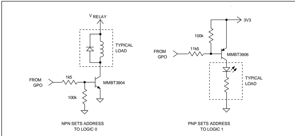
Figure 11. Output drivers polarity sets 5171 address during reset.
