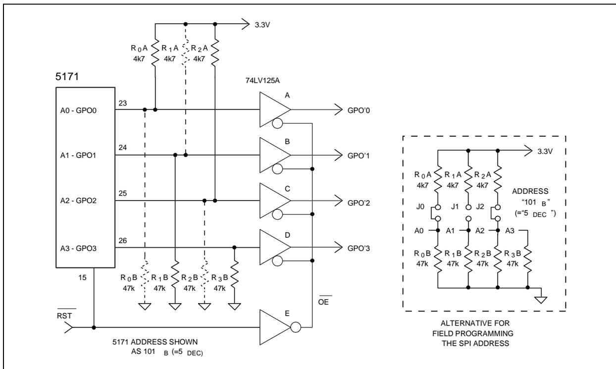
Figure 12. 5171 device addressing with buffered GPO outputs.
