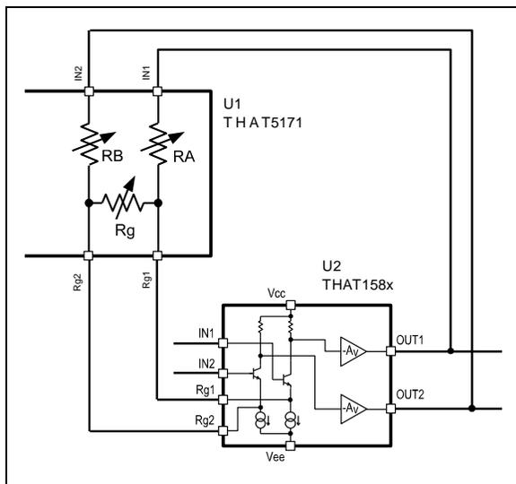
Figure 2. Analog portion of 5171 connected to a 158x.
