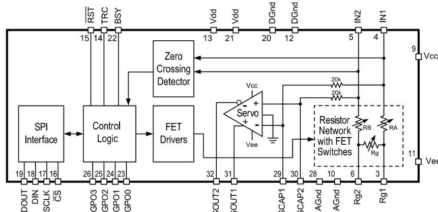
Figure 1. THAT 5171 Block Diagram
