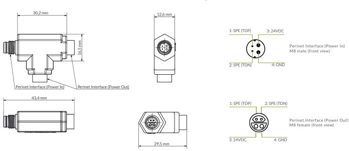
This periSWITCH 3-port switch facilitates the series connection of multiple sensors and/or actuators.
