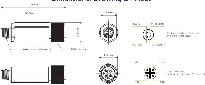
This periNODE smart adapter connects directly to sensors with Pt100 3-wire signal output and M12 A-coded 4-pin connectors.
