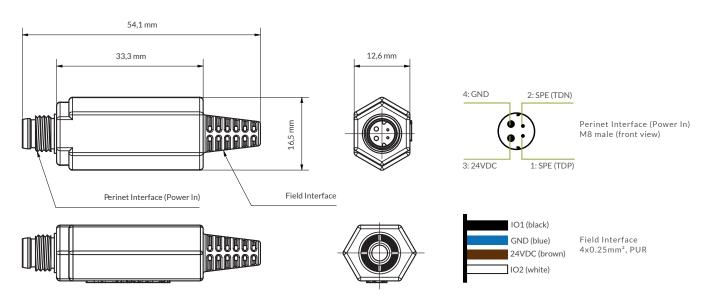
This periNODE smart adapter has 2 in-/output channels and connects directly to sensors or actuators with 24V GPIO via a 4\*0.25mm² cable. It turns the analogue, passive sensor or actuator into a smart, active network participant that communicates via ethernet with any IT-system or data hub. periNODE permits the configuration of data communication intervals to meet user-specific demand, thereby reducing network traffic and redundant data collection.
