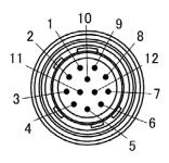
Output connector HIOKI ME15W of current sensors HIROSE ELECTRIC CO., LTD. HR10A-10P-12P(74)
