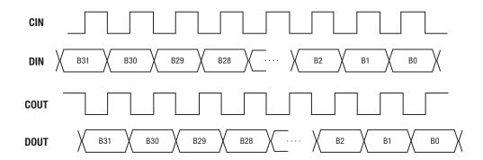
The serial command is transmitted with MSB first, DIN is latched at the rising edge of CIN clock. COUT and DOUT are re-generated for the next RGB LED. COUT is inverted from CIN. When 32 consecutive 0's are encountered, the next 1 is expected to start a 32-bit command, i.e., FLAG [2:0]=111. When FLAG [2:0]=111, then DIMMING, BLUE, GREEN and RED fields are latched respectively. While the current 32-bit command is got, IC passes remaining command bits to the next RGB LED.
