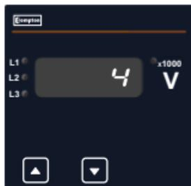
This screen is used to set the system type. System type “3” for 3 phase 3 wire & “4” for 3 phase 4 wire system.
