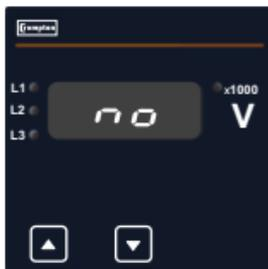
Pressing the "↓" key will accept the display value and exit from set up and enter into measurement mode.
