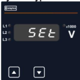
This screen will only appear following the edit of system type. If system type is to be edit again, Pressing the “ $\uparrow$  up” key will scroll between “3” for 3 phase 3 Wire and “4” for 3 Phase 4 Wire.
