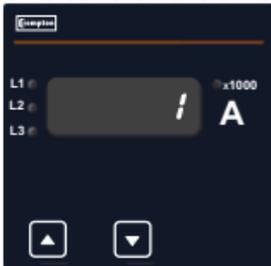
This screen is used to set Current transformer secondary value. "1" for CT secondary 1A and "5" for CT secondary 5A. pressing "↓" down key accepts the present value and advances to the Auto Scroll option in case of DGU -3A and for DGU -1A it will exit from setup and goes to measurement screen.
