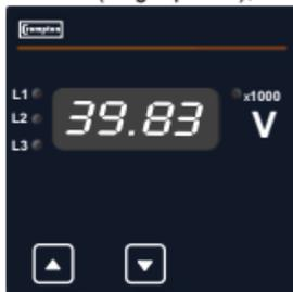
Pressing the “ $\downarrow$ ” key accepts the present value and advances to the “PT Secondary” selection menu(See Section 3.1.4) for DGU -3V and 1V.
