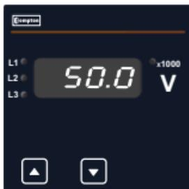
Pressing the "↓" key accepts the present value and advances to the "Auto scroll" selection menu (See Section 3.1.6) for 3V. In case of DGU 1V it will exit from set up menu.
